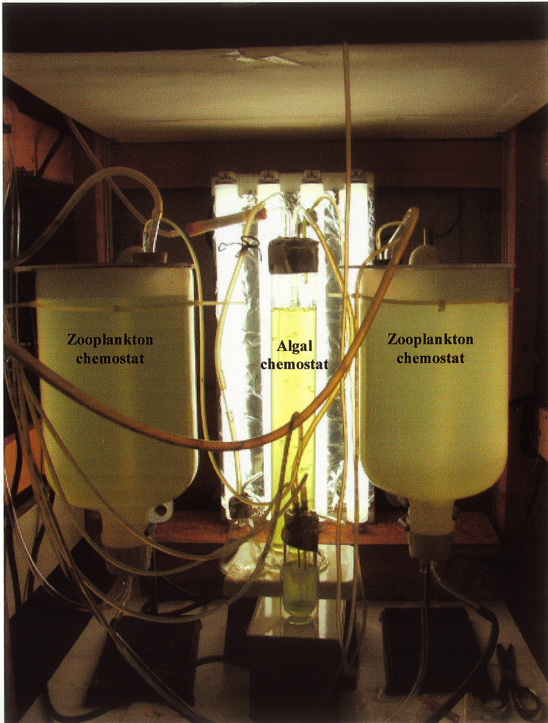
Figure 2. The algal/zooplankton chemostat used for culturing Daphnia pulicaria and algae for the feeding experiment.
