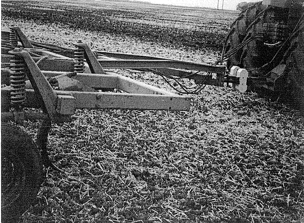
Fig. 14 The dynamometer used for measuring draft force requirement. (The dynamometer was fitted between the implement and the tractor).
