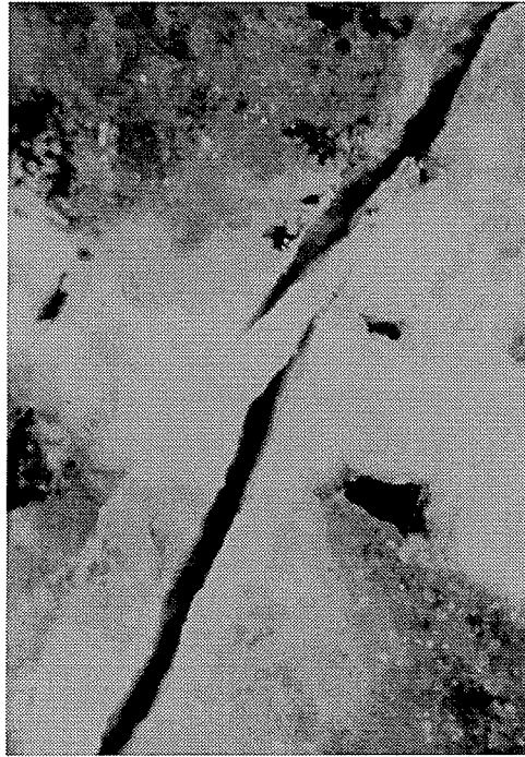
Figure 4.11: Photo of step-out fractures in Cold Spring granite.
