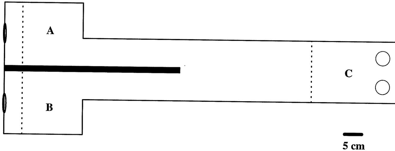
**Figure 4.1** Top view of a two-way choice apparatus for behavioural experiments. The diagram is proportional to the actual size. The trough is arbitrarily labelled as sections A, B, and C for the convenience of illustration. Two circles in section C indicate positions of two water outlets. Dashed lines indicate the positions of three perforated plastic plates. Two elliptical circles indicate water inlets. Black bar in the middle of trough indicates the plexiglass wall. Bar=5 cm.
