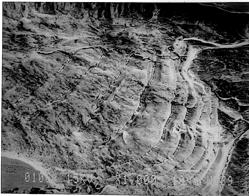
Fig.4-19 SEM micrograph of the wear track with fatigue bands on the delaminated place after 4kg, room temperature test (as-deposited coating)
