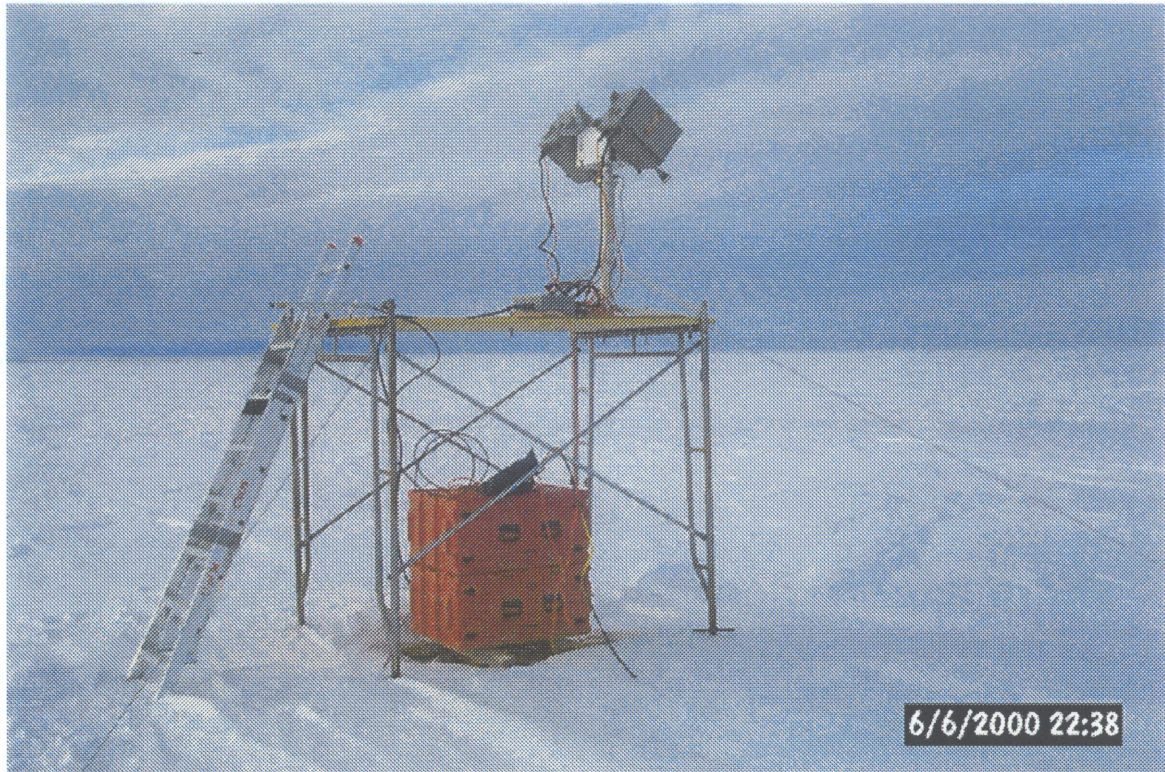
Figure 3.2. SBR system at fixed deployment site.
