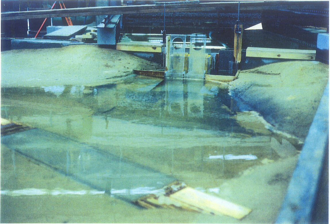
Figure 4.7 Fixed point gauge to the right of the powerhouse used for measuring water surface elevations by the intake and beside the draft tube.
