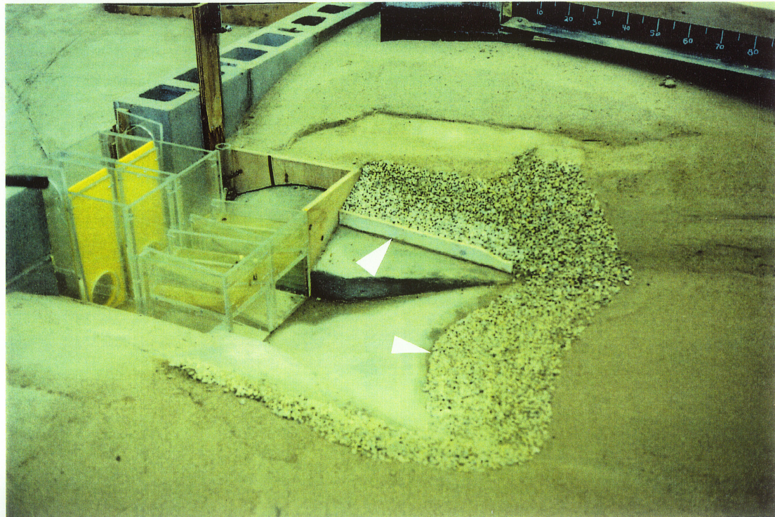
Figure 5.18 Retaining wall and riprap (less than 1 m diameter, prototype scale) to mitigate erosion in the tailrace.
