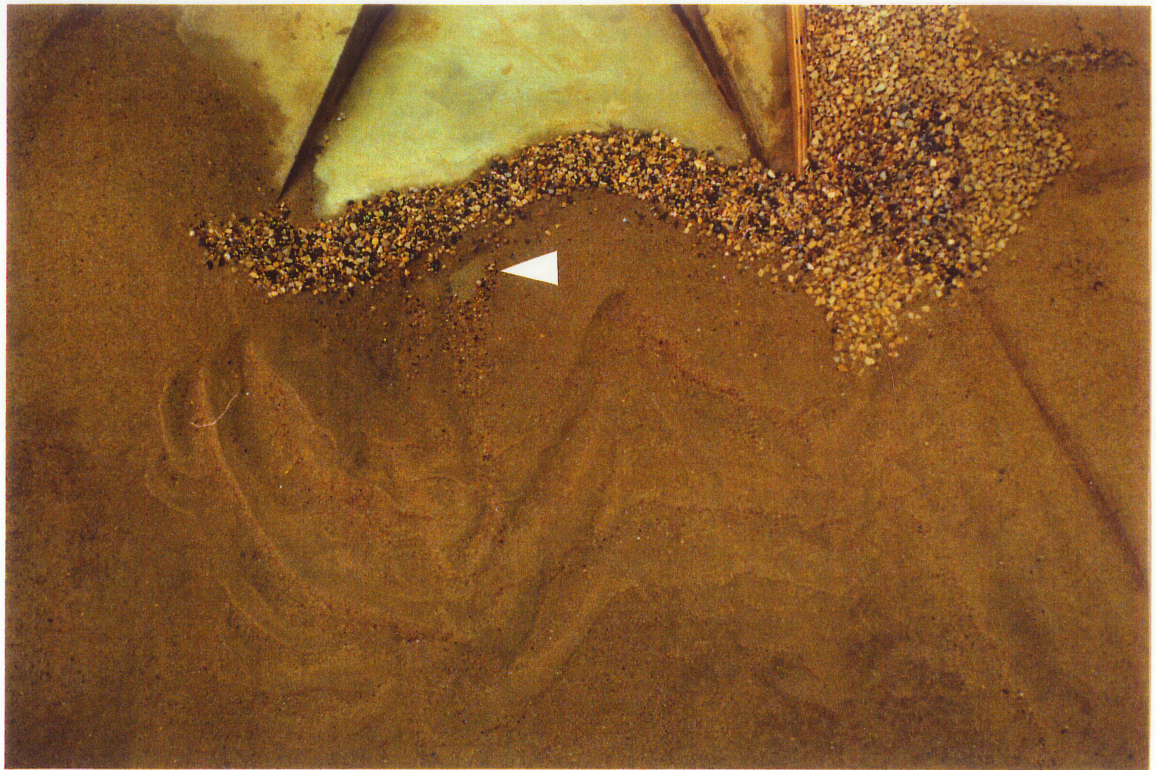
Figure 5.23 Erosion of the overburden Removal Scheme DOB1, in spite of the riprap.
