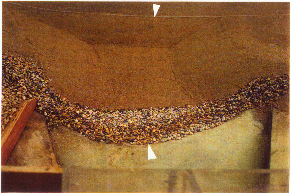
Figure 5.24 Overburden Removal Scheme DOB2 where the overburden is removed to two-thirds the distance to the downstream cofferdam to an invert of 231 m, with riprap at the leading edge.
