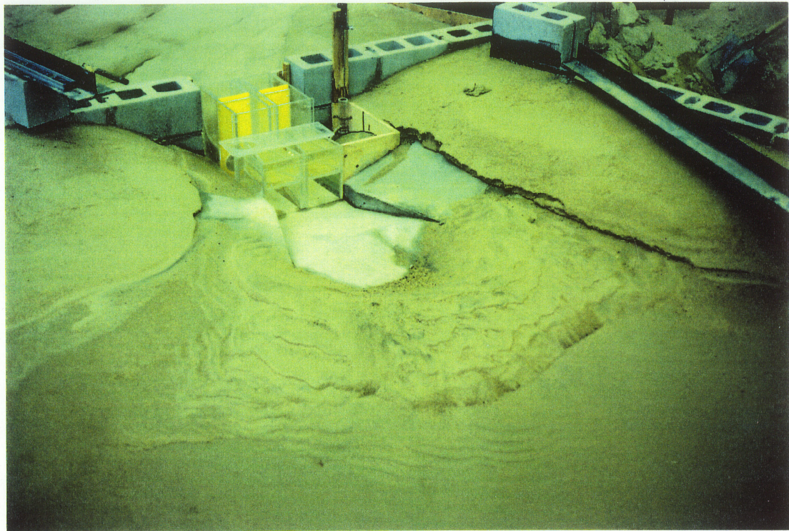
Figure 5.17 Erosion of the overburden downstream of the powerhouse.
