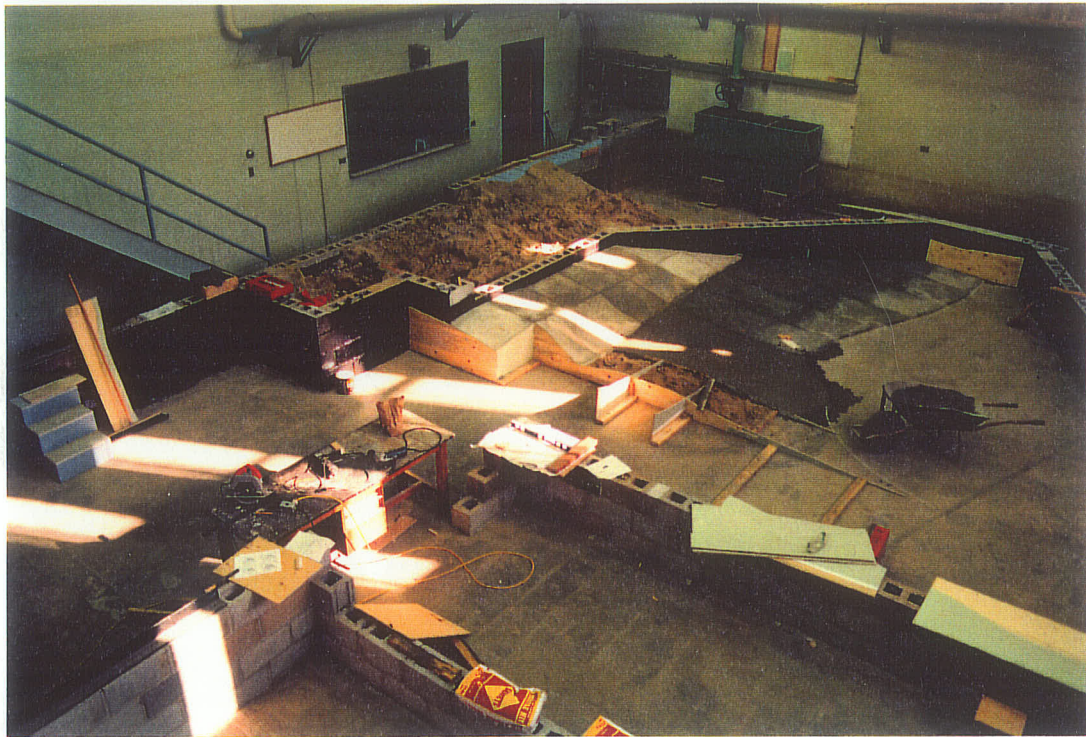
Figure 4.1 Construction of the physical model for the Notigi Generating Station showing formation of bedrock using templates, sand, and concrete.
