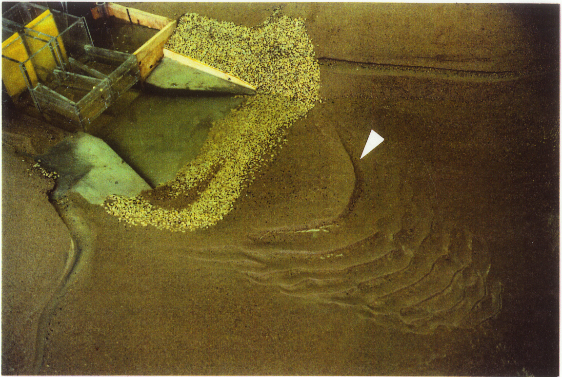
Figure 5.19 Erosion of the downstream overburden, even with riprap in place.
