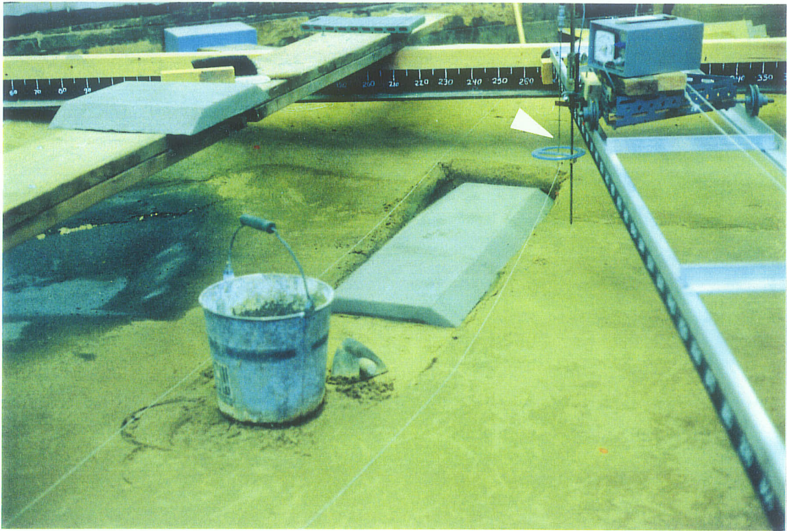
Figure 4.9 View of the point gauge and mini-flow current meter mounted to the instrument wagon on a mobile bridge.
