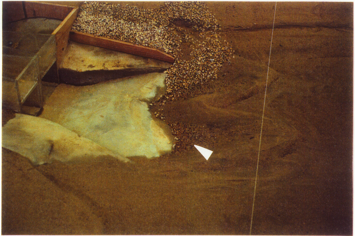
Figure 5.21 Erosion of the overburden Removal Scheme DOB1.
