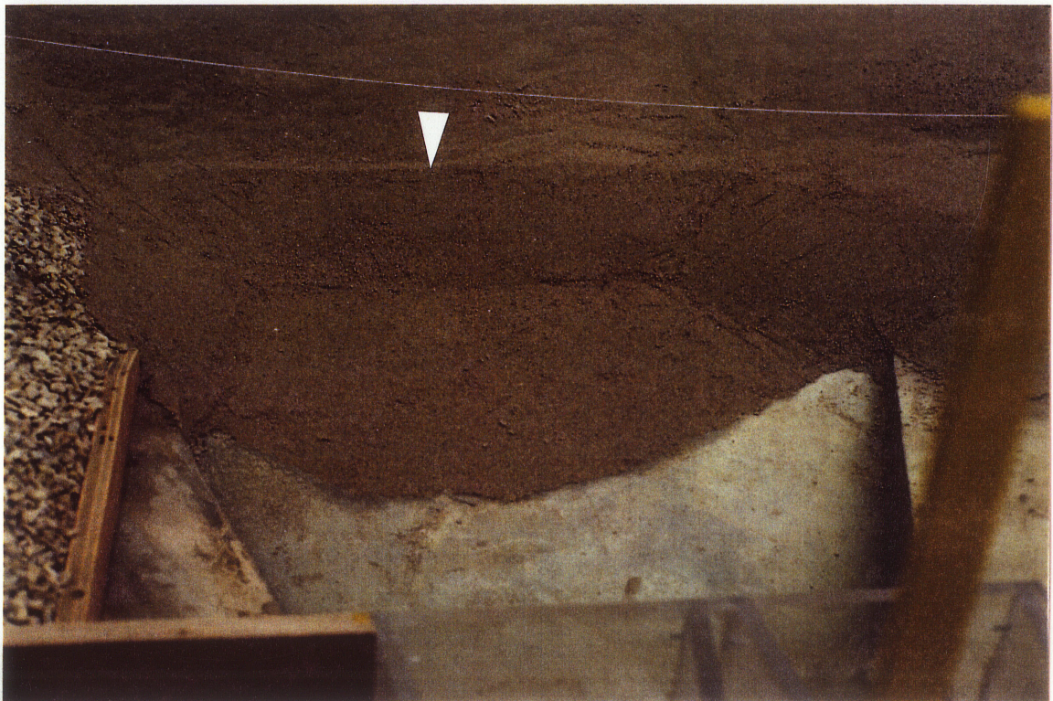
Figure 5.20 Looking downstream from the powerhouse at the overburden Removal Scheme DOB1 where the overburden is removed to one-third the distance to the powerhouse to an invert of 231 m (no riprap).
