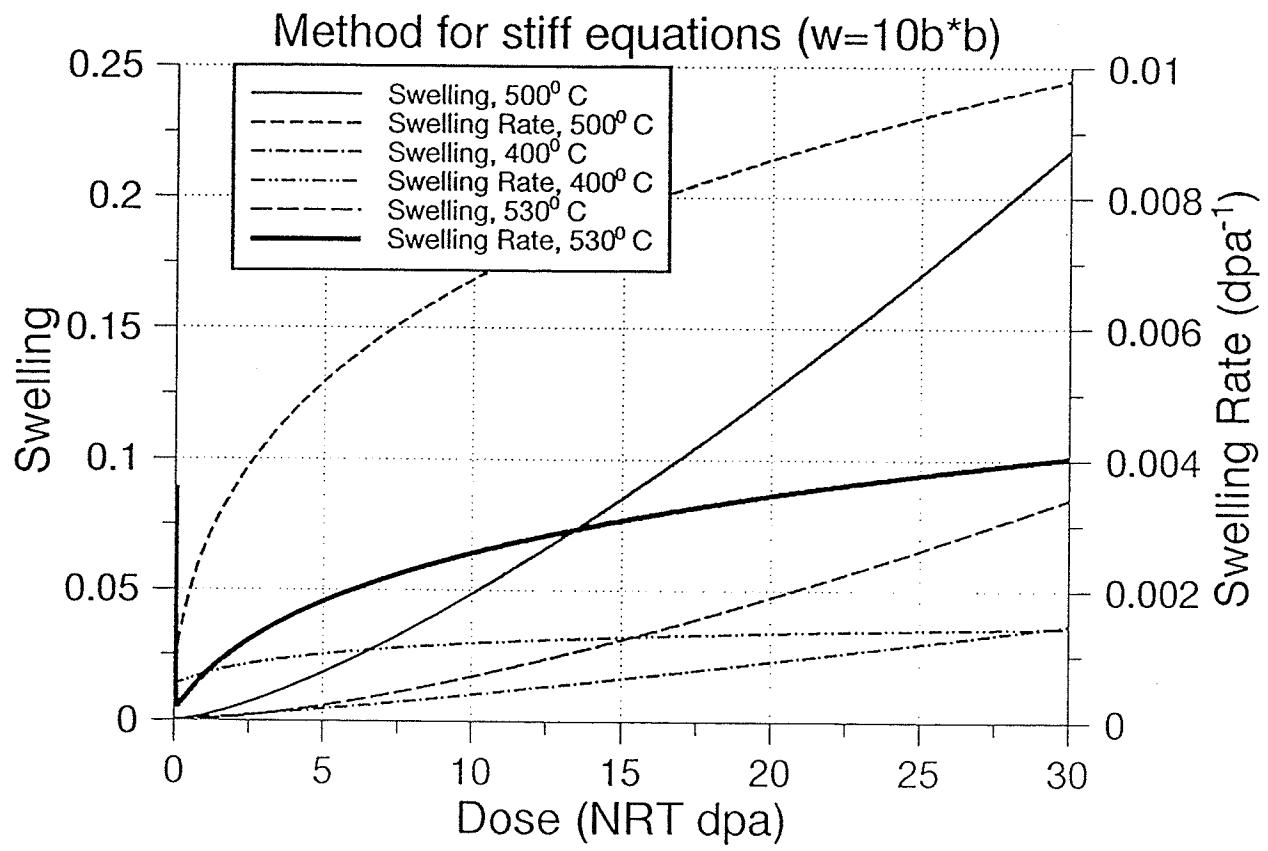
Fig.4.7 Dose dependence of calculated void swelling using the method for stiff set of equations. Parameters are the same as the ones used to derive figures 4.4 and 4.5.
