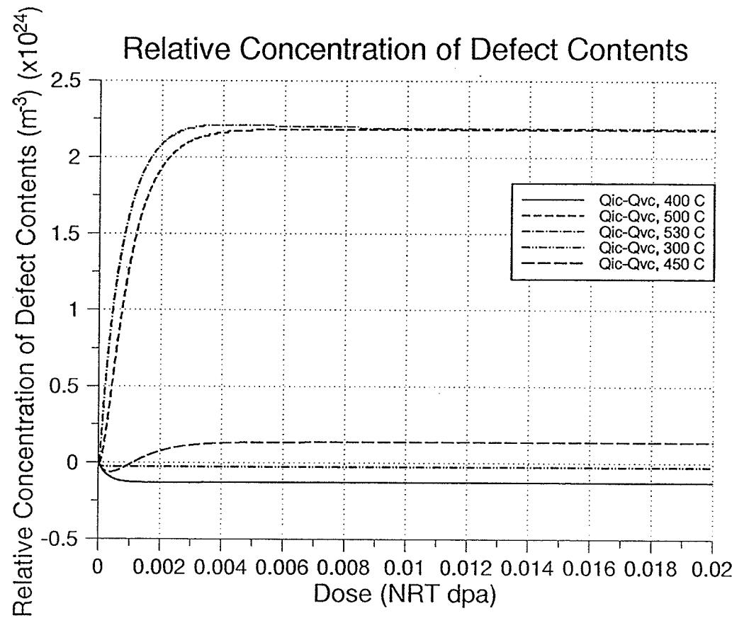
Fig. 4.3 Dose dependence of calculated difference between interstitial concentration in PICs and vacancy concentration in PVCs. Parameters are the same as the ones used to derive figs. 4.1 and 4.2.
