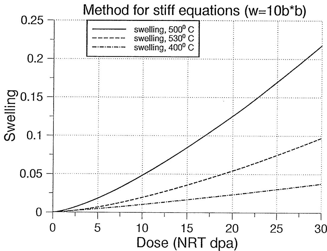
Fig.4.5 Dose dependence of calculated void swelling for 316 stainless steel in different temperature regions: low swelling (400°C), swelling peak (500°C) and post swelling-peak(vacancy evaporation from voids) (530°C). The material parameters are listed in the appendix B.
