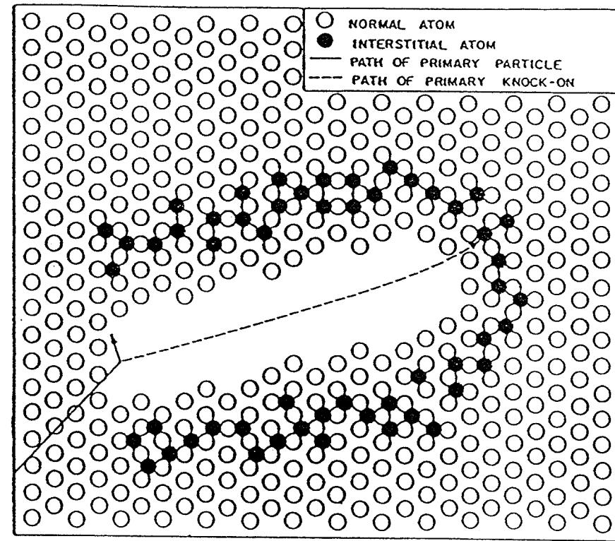
Fig.1.2 The collision cascade shown schematically (after M.W. Thompson[13]).
