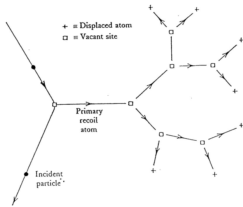
Fig.1.1 The multiple displacement in the core of cascade region (after M.W. Thompson [13]).
