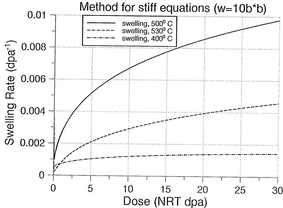
Fig.4.4 Dose dependence of calculated void swelling rate for 316 stainless steel in different temperature regions: low swelling ( $400^\circ\text{C}$ ), swelling peak ( $500^\circ\text{C}$ ) and post swelling-peak(vacancy evaporation from voids) ( $530^\circ\text{C}$ ). The material parameters are listed in the appendix B.
