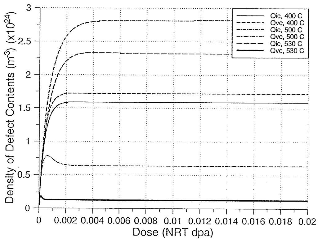
Fig.4.2 Dose dependence of calculated average total defect contents in the PICs and PVCs for 316 stainless steel in different temperature regions: low swelling ( $400^\circ\text{C}$ ), swelling peak ( $500^\circ\text{C}$ ) and post swelling-peak (vacancy evaporation from voids) ( $530^\circ\text{C}$ ). The material parameters are listed in the appendix B.
