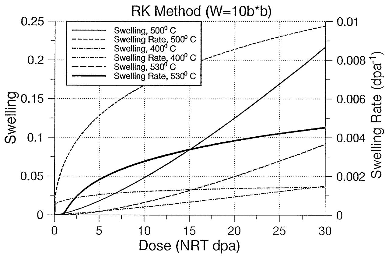
Fig.4.6 Dose dependence of calculated void swelling using Runge-Kutta method. Parameters are the same as the ones used to derive figures 4.4 and 4.5.
