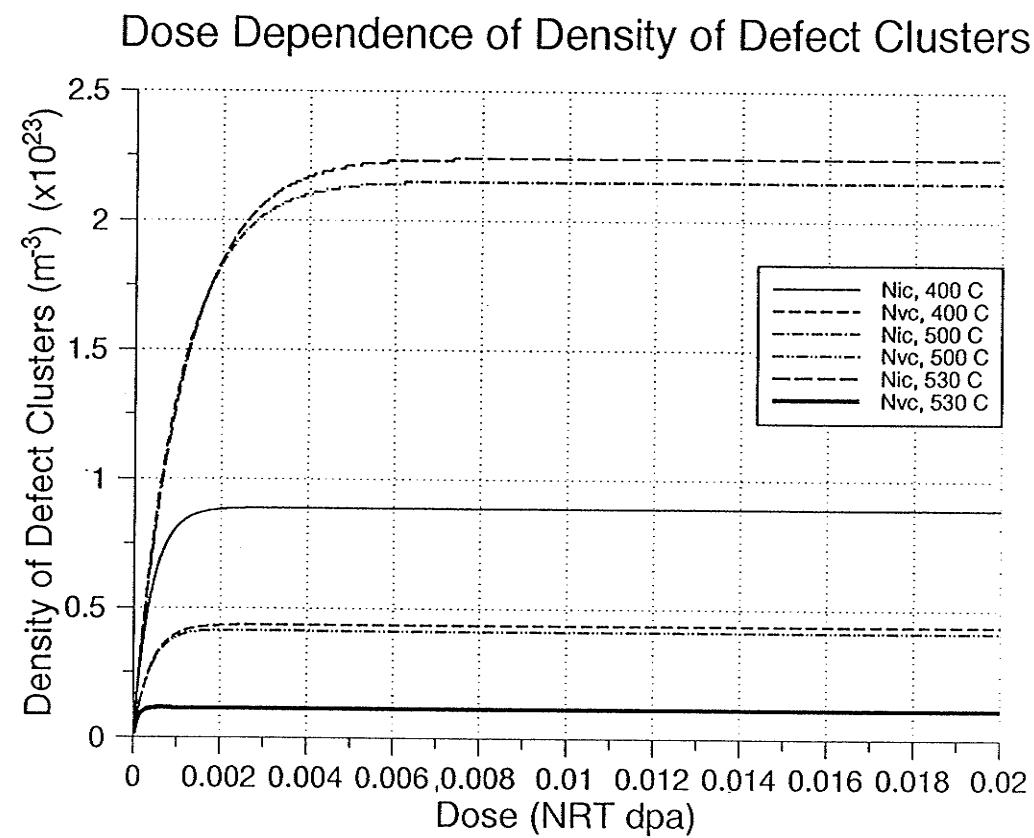
Fig.4.1 Dose dependence of calculated number densities of the PICs and PVCs for 316 stainless steel in different temperature regions: low swelling (400°C), swelling peak (500°C) and post swelling-peak(vacancy evaporation from voids) (530°C). The material parameters are listed in the appendix B.
