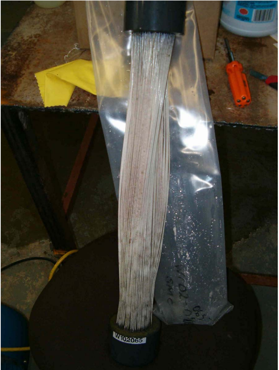
Figure 23: Membrane with mold growth. Transport packaging in back
