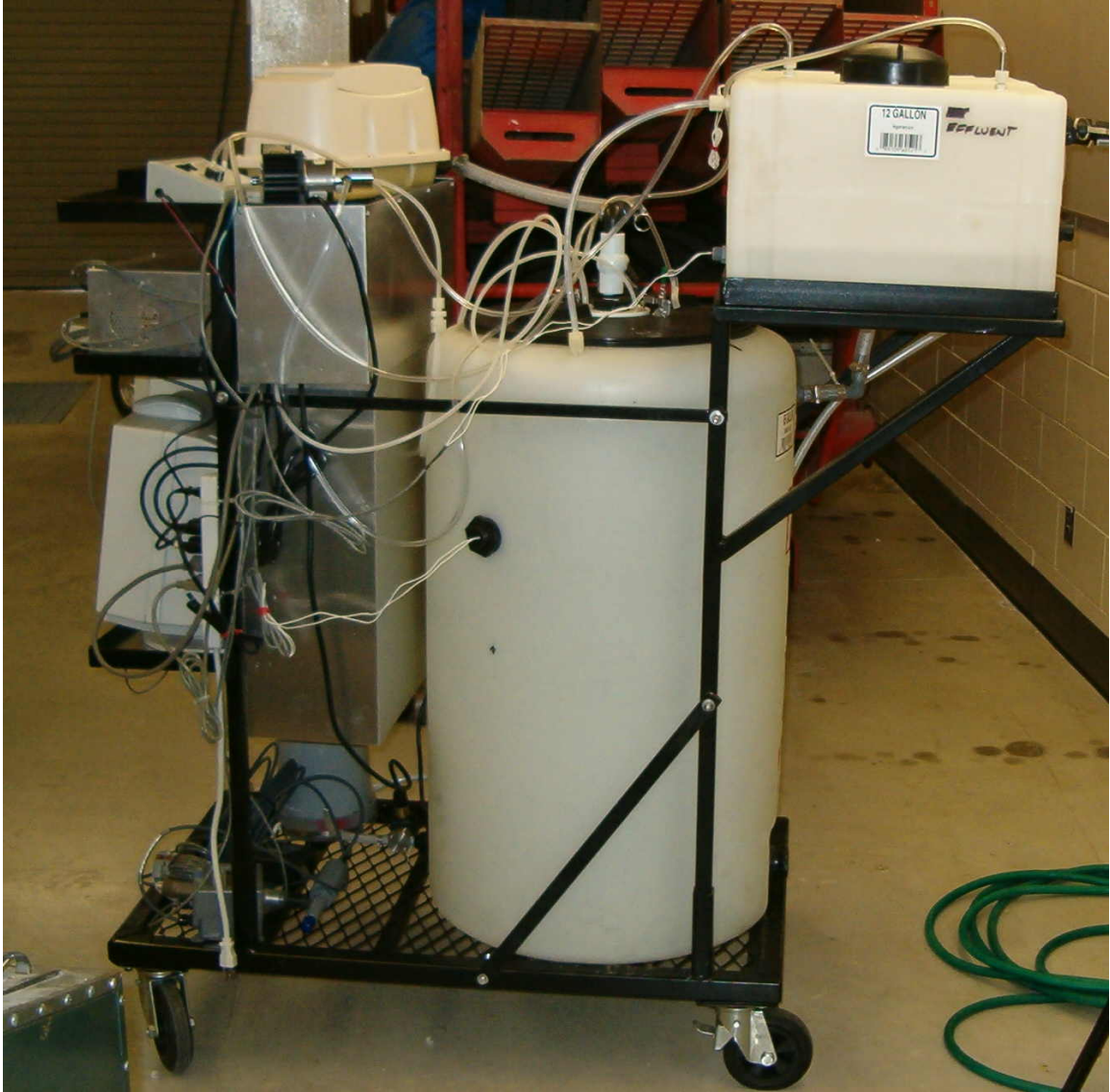
Figure 12: MBR Pilot System (right side)
