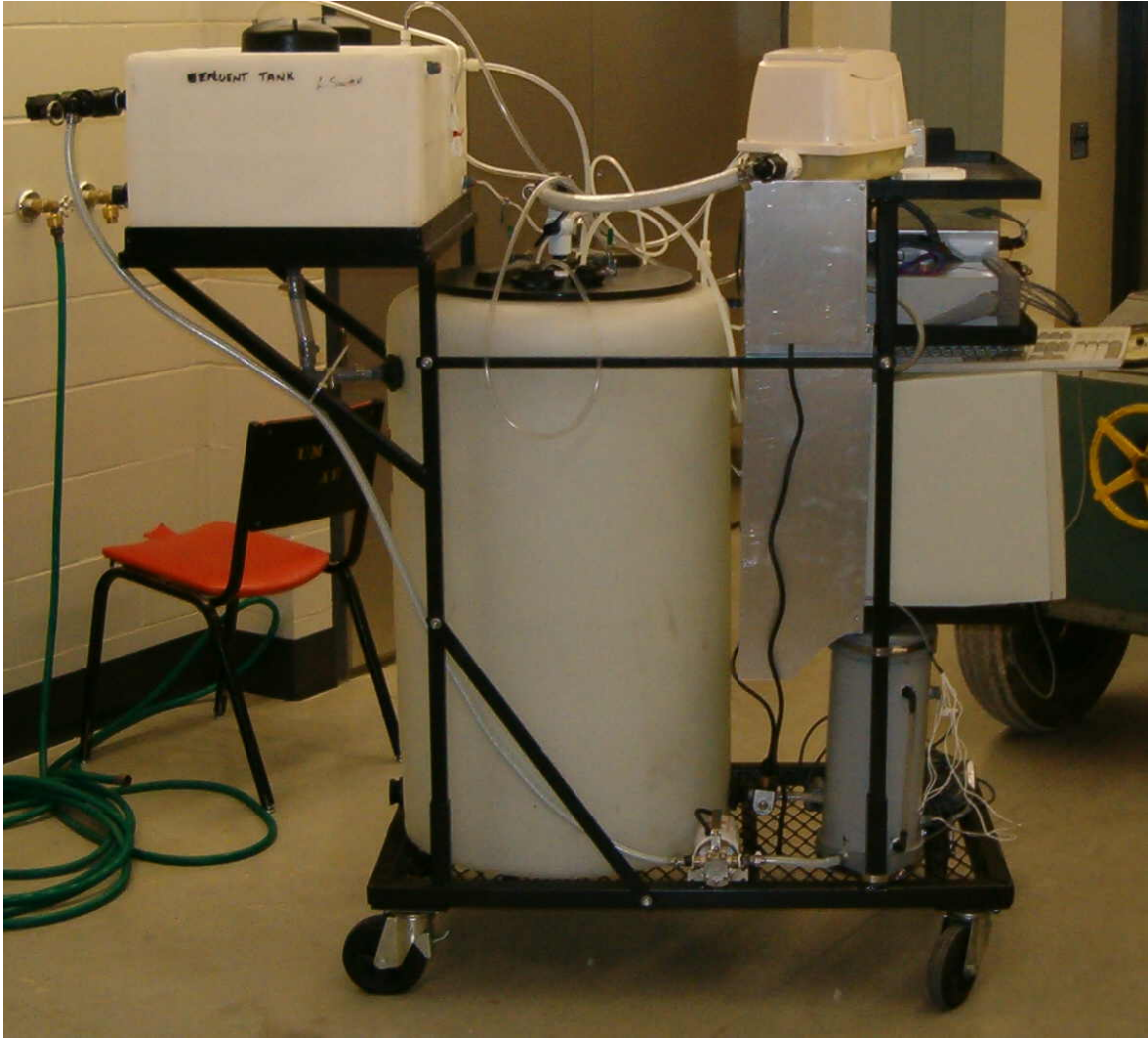
Figure 11: MBR Pilot System (left side)
