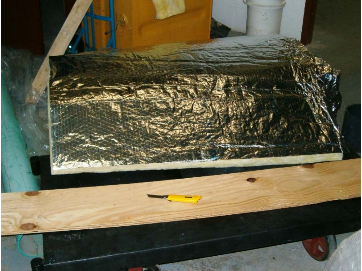
Figure 20: Reflective Insulation for Feed Water Piping.
