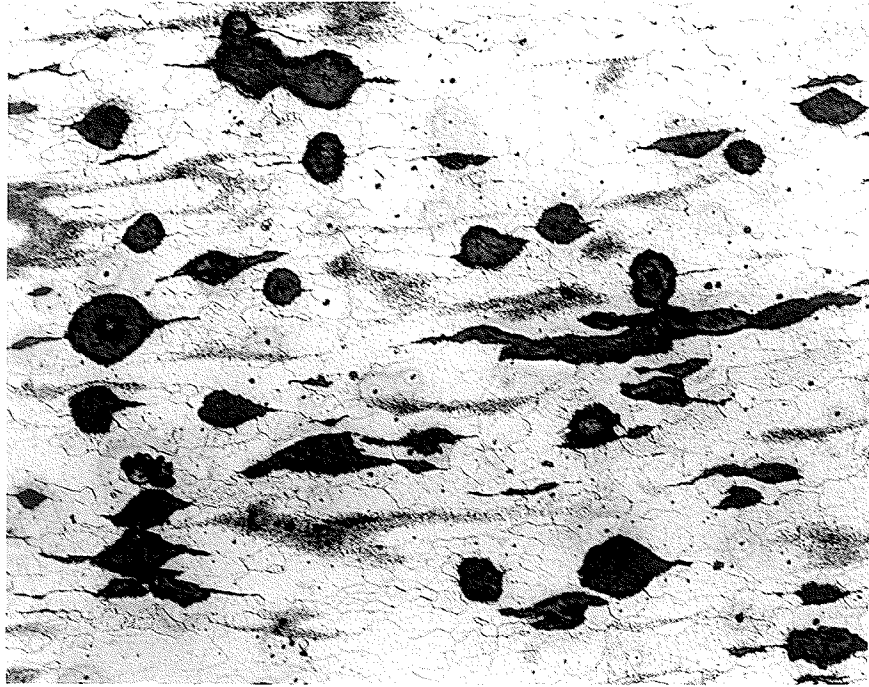
Figure 23 Optical micrograph of a longitudinal section of as received material tested in compression at 750°C. 210X, etchant 2% nital.
