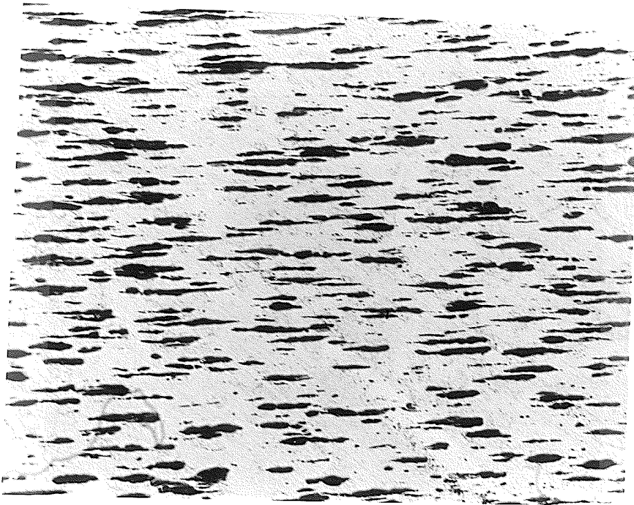
Figure 68 Optical micrograph of a longitudinal section of material hot swaged at 934°C from 0.56 inches in diameter to 0.332 inches in diameter and cold swaged at room temperature from 0.332 inches in diameter to 0.20 inches in diameter. 52.2X, unetched.
