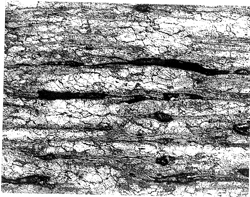
Figure 59 Optical micrograph of a longitudinal section of material swaged at 850°C from 0.5 inches in diameter to 0.2 inches in diameter, in the untested condition. 210X, etchant 2% nital.
