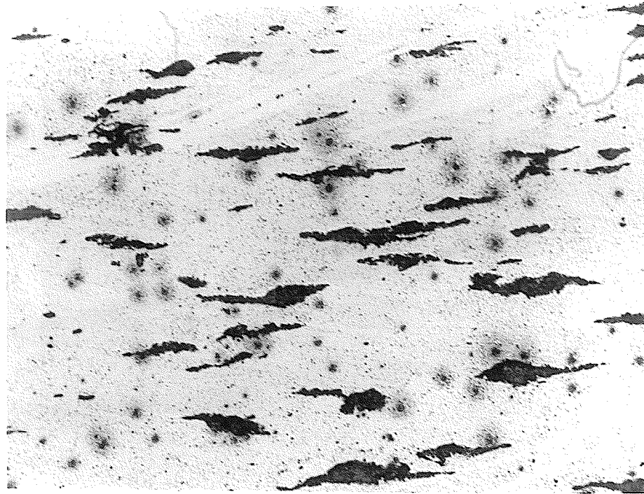
Figure 64 Optical micrograph of a longitudinal section of material hot swaged at 934°C from 0.56 inches in diameter to 0.448 inches in diameter and cold swaged at room temperature from 0.448 inches in diameter to 0.322 inches in diameter. 210X, unetched.
