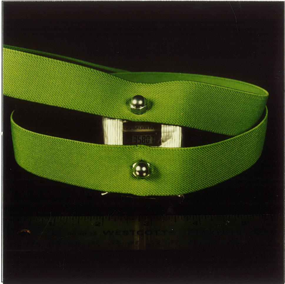
Figure 1. Digital pedometer (DIGI-WALKER MINI, EM-201, Yamax Corp., Yokohama) modified for cow use by encasing it in plexiglass and attaching straps.
