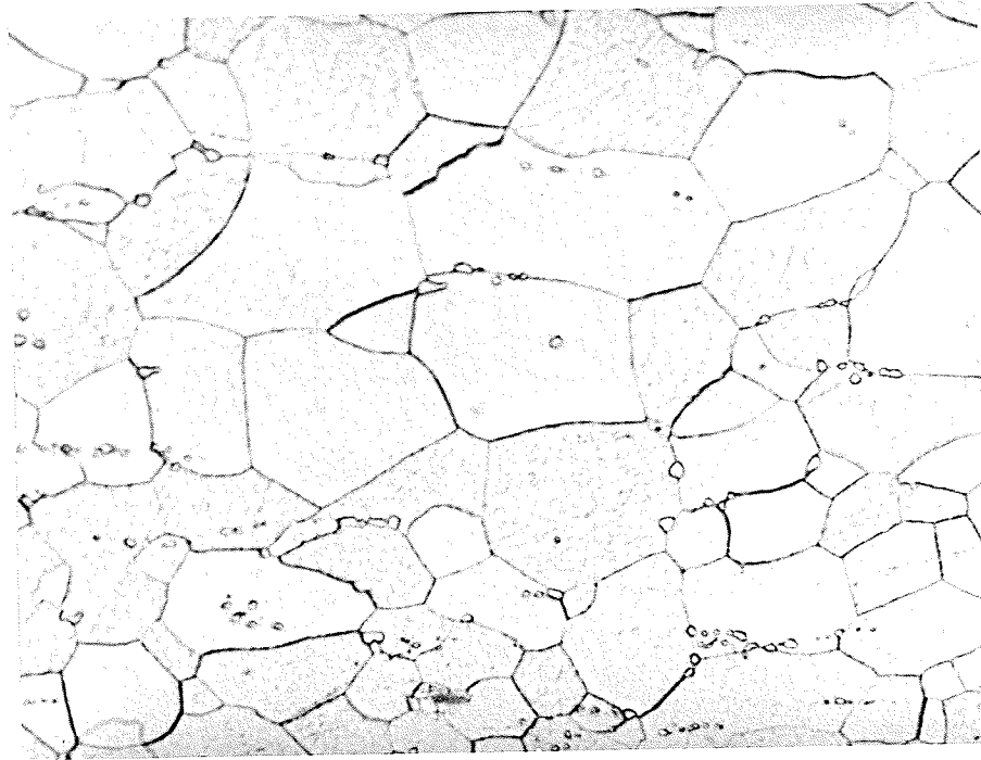
FIGURE 10 Liquid Withdrawal Tube Micro Structure (1322X)
