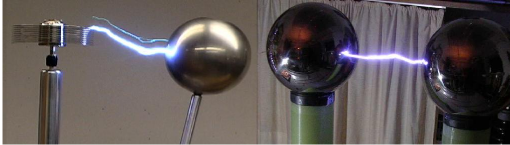
Figure 2.1: Electric Breakdown a) Between HV Sphere and Electrode, b) Between Sphere and Sphere. Adopted with Modifications from [2], [3]. Photos ©2004 University of Michigan Demonstration Laboratory, and ©2006 Kurt Schraner Respectively. Both Images Used by Permission.
