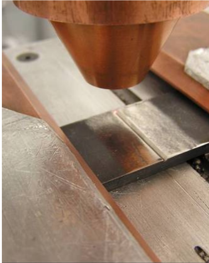
Figure 3: Close-up of laser welding nozzle and v-notch test specimen.
