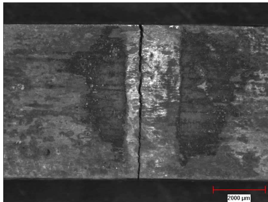
Figure 121: Crack along fusion zone, 0.3% strain René 80
