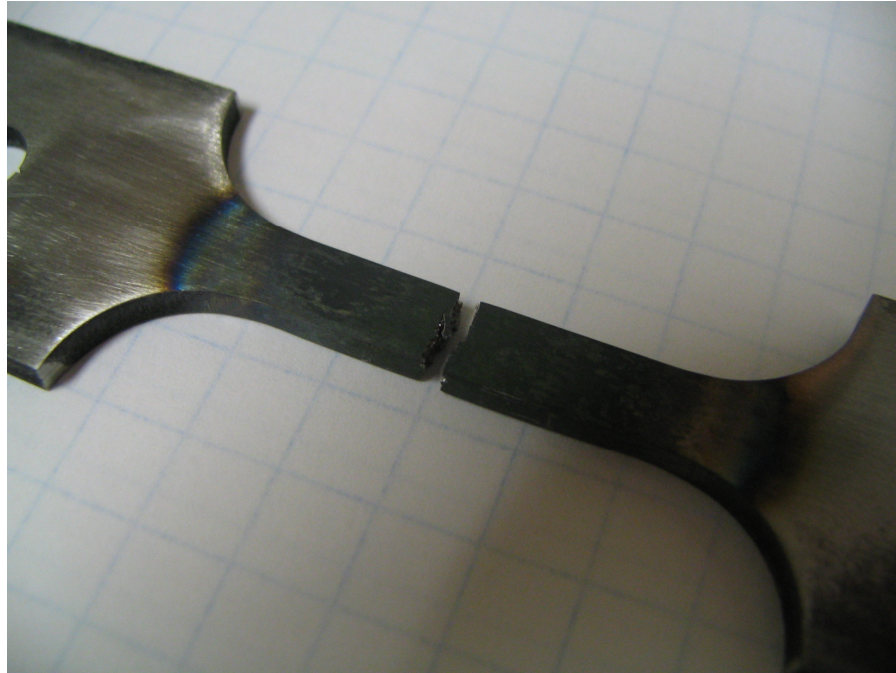
Figure 100: Fractured René 80 TMF specimen, 0.2% strain
