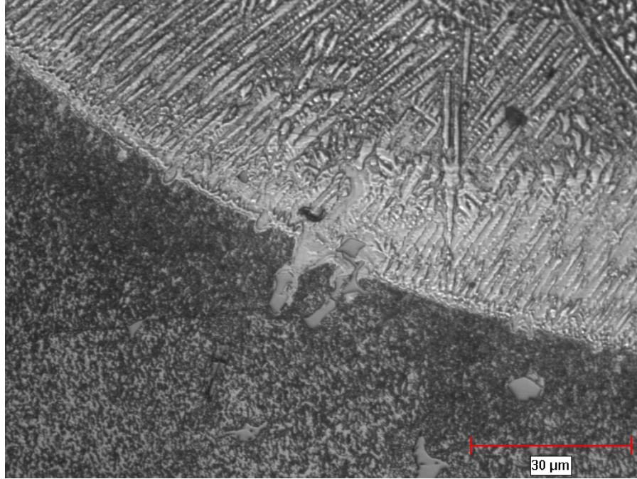
Figure 39: Optical micrograph of the weld fusion zone interface in René 80
