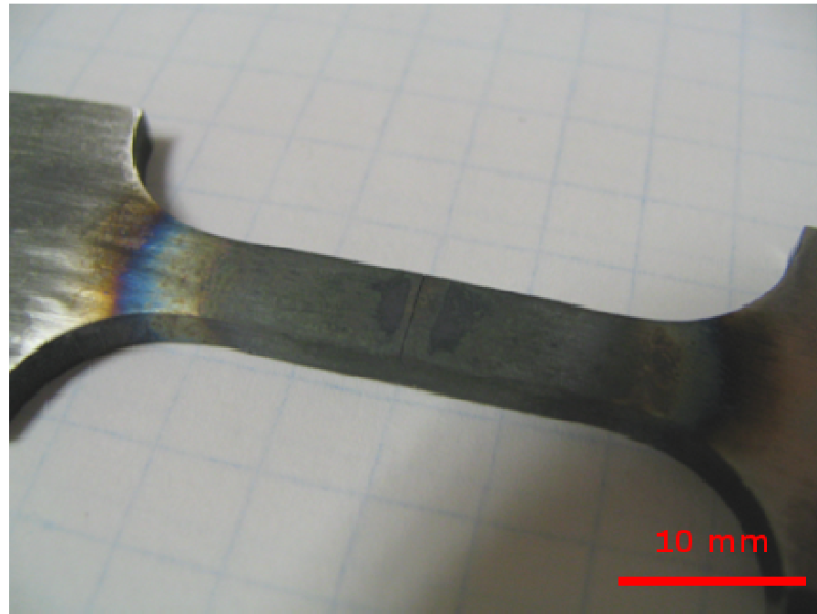
Figure 120: 0.3% strain René 80 TMF specimen
