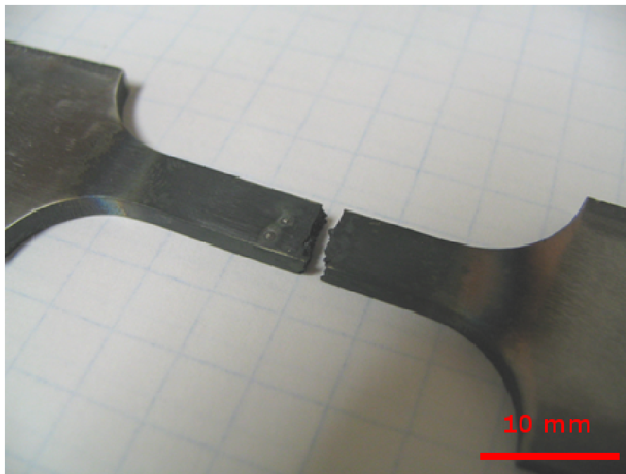
Figure 110: Fractured 0.25% strain René 80 MF specimen
