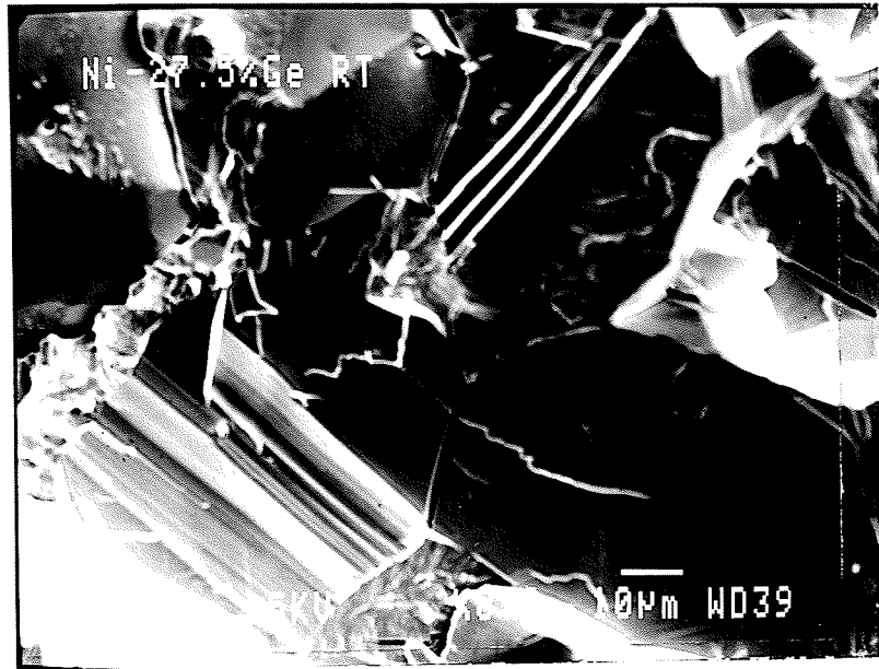
Fig 4.33 Ni-27.5 at% Ge failed at 21°C (850X)
