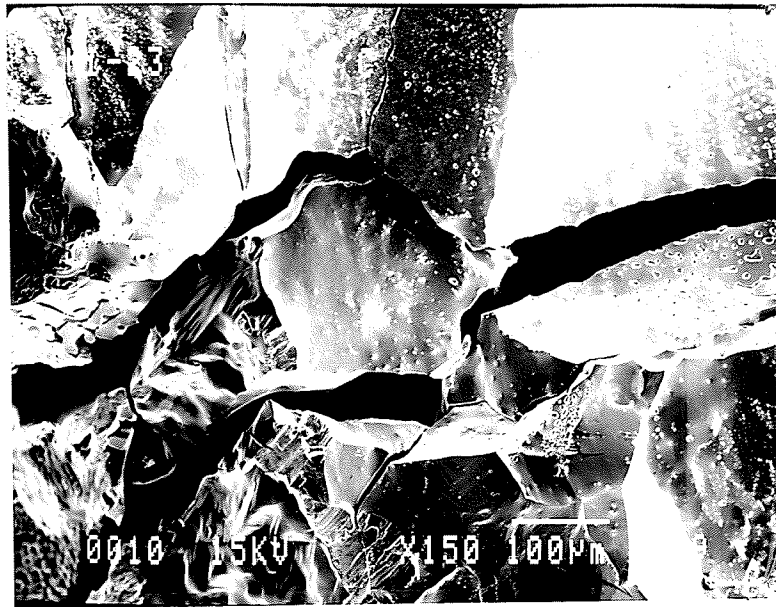
Fig 4.25 Ni-23.5 at% Ge failed at 400°C (150X)
