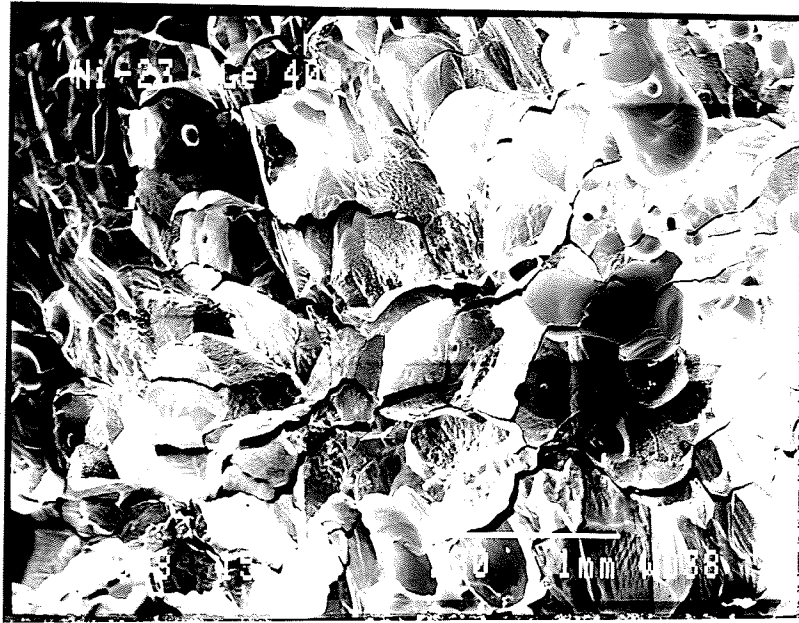
Fig 4.23 Ni-23.5 at% Ge failed at 400°C (30X)
