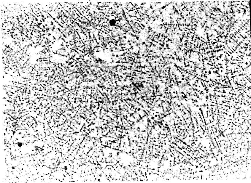
Fig 4.1 Ni-20 at% Ge Homogenised (50X)
