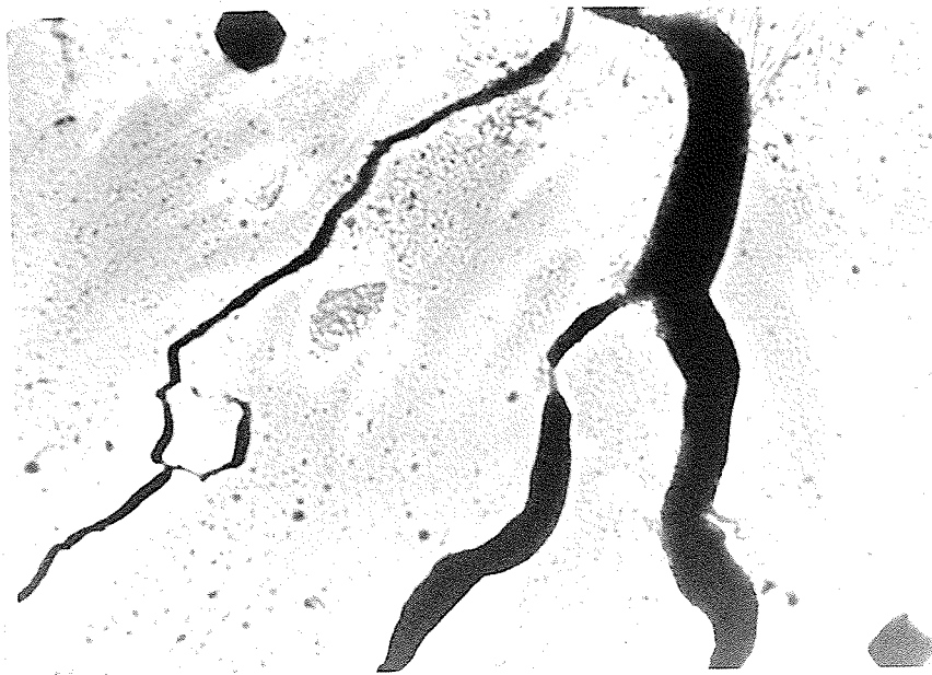
Fig 4.39 Ni-25.0 at% Ge deformed at 700°C (50X)
