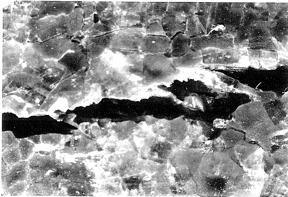
Figure 4.42 Photographs of the buckling and shearing processes which the rock bridges from figure 4.41 undergo. The final result is a single macroscopic crack. Loading is from left to right and magnification is ten times.
