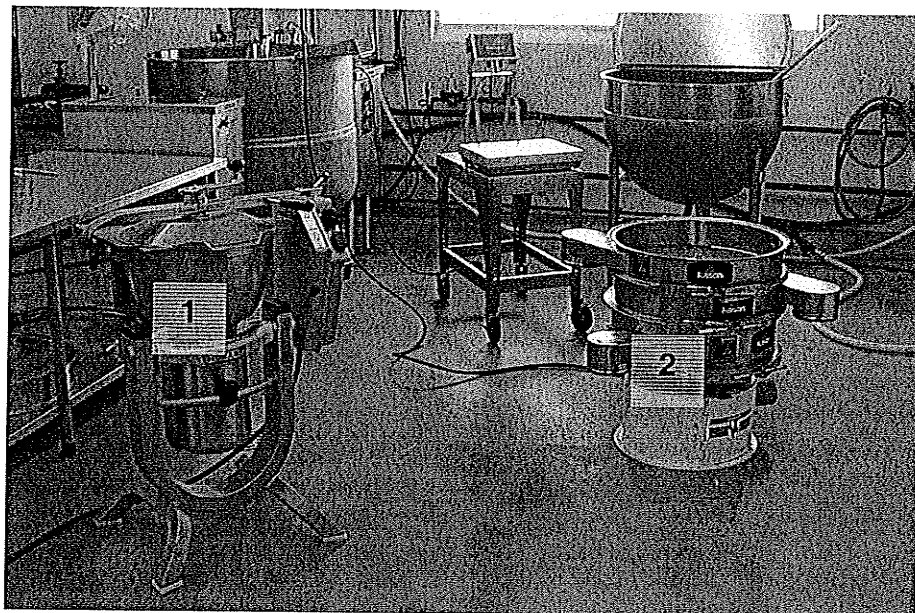
Fig. A1-7. Separation pilot process. (1) Hobart cutter mixer used to thresh the dry press cake. (2) Vibratory screen separator used to separate seeds from the pulp.
