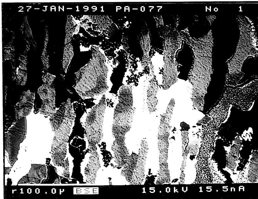
Fig. 4.3-2. BSE images of Helikon pollucite. a) Cs-rich pollucite next to a large, lightly zoned mica grain. At photo center, an adularia grain with increasing Rb from core to rim. b) Top half is an area of mica/quartz intergrowth, bottom half is a mica/pollucite intergrowth, grading to area of pollucite.
