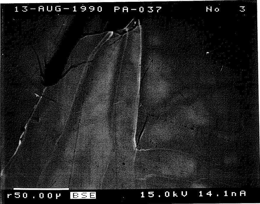
Fig. 4.4-3. BSE images of Morrua pollucite. a) and b) A slight heterogeneity of "homogeneous" pollucite: incipient development of Na-enriched and Cs-enriched domains.
