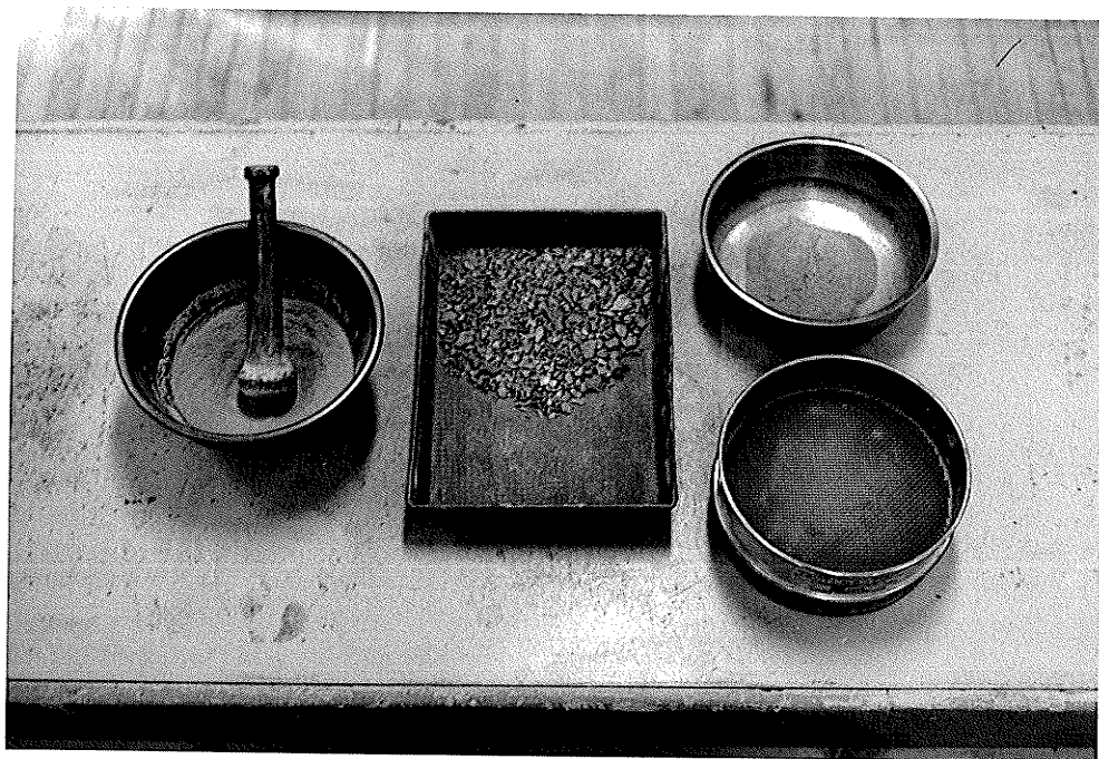
Photograph B-1: Mortar and Pestle Used for Breaking Up Aggregations of Soil Particles for Clays Property Tests -- Pestle Also Used in Clay Mortar Mixing and in Breaking Up Hardened Lime-Sand Mortar for Remix Mixes
