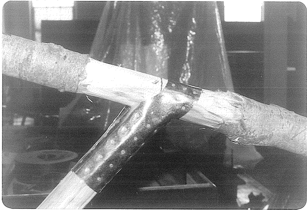
Fig. 2-3: Top Chord / Web Member Connector
