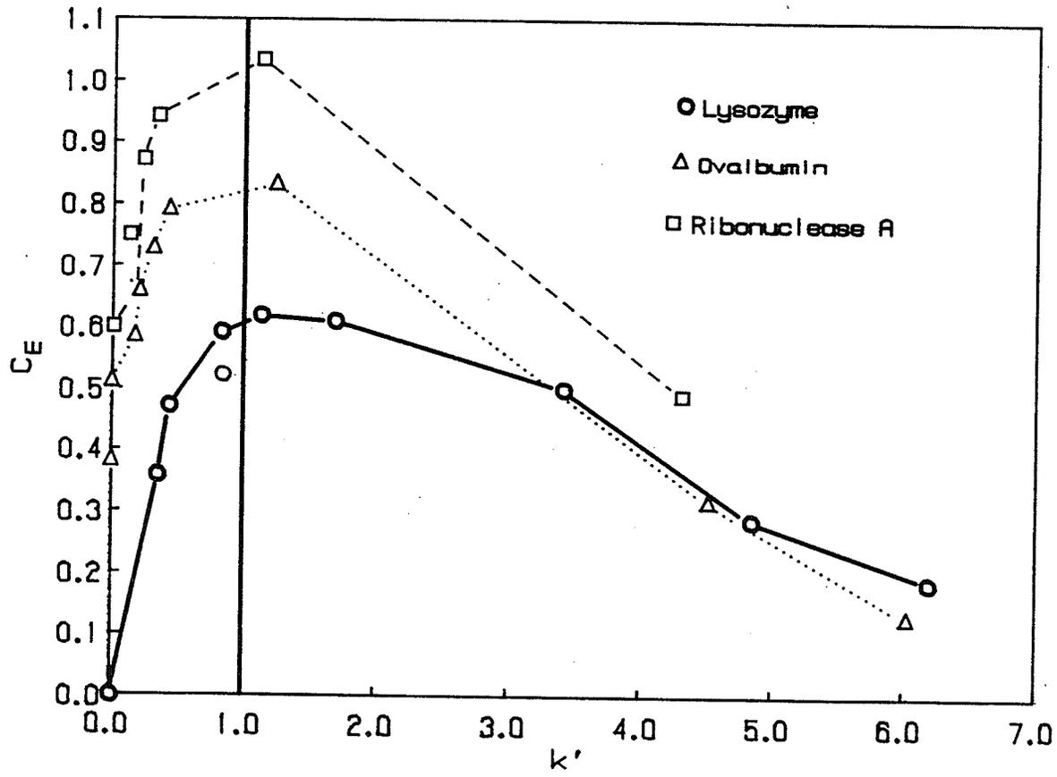
Figure 3. The effect of initial ammonium sulfate concentration on the elution environment of lysozyme, ovalbumin and ribonuclease.
