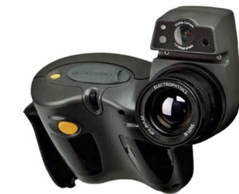
FIGURE 2.5: The infrared whole-field thermography camera used in the experiment.
