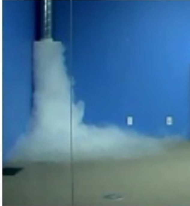
FIGURE 2.6: DV flow pattern visualized by smoke test.
