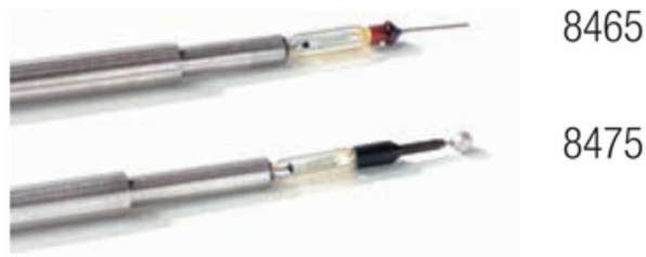
FIGURE 2.3: The low-temperature thermal anemometers: TSI 8475 omni-directional hot sphere and TSI 8465 windowless probes used for measurements of the mean air velocity and fluctuations.
