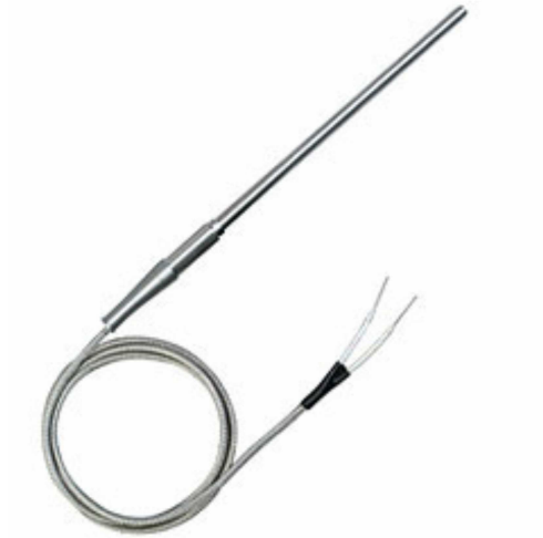
FIGURE 2.4: The RTD probe used in the experiment.
