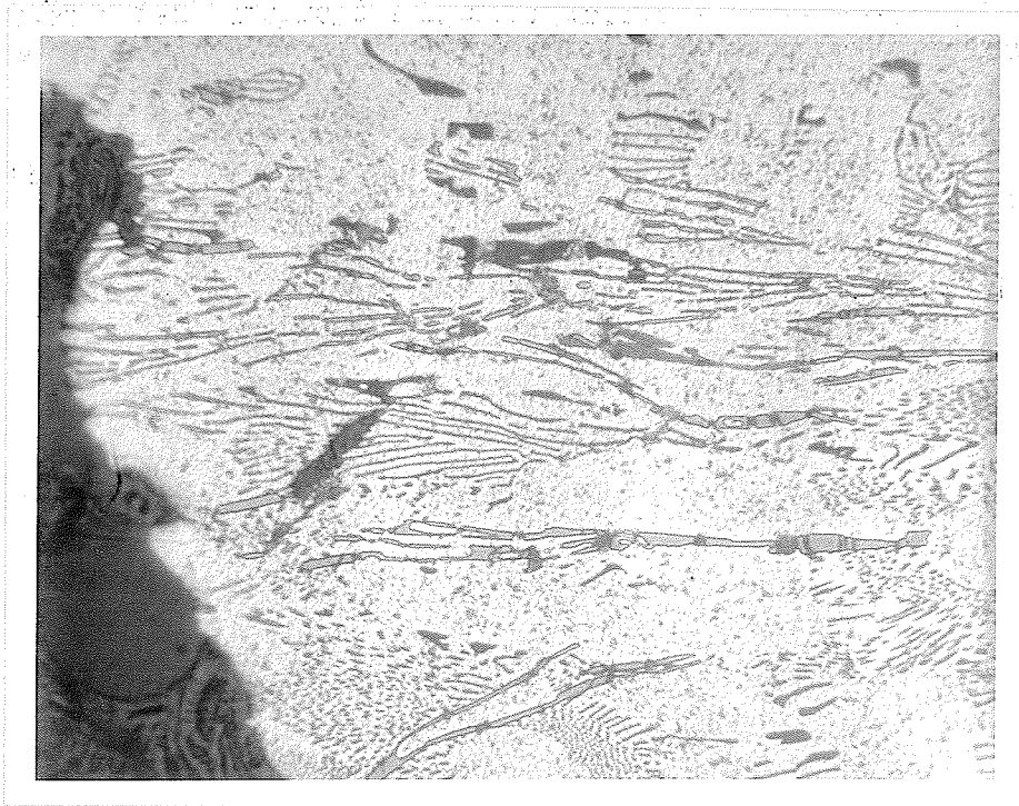
Fig. 45 Al-4.6%Ni showing fracture through a fibrous region indicating that fiber strengthening occurs X455.
