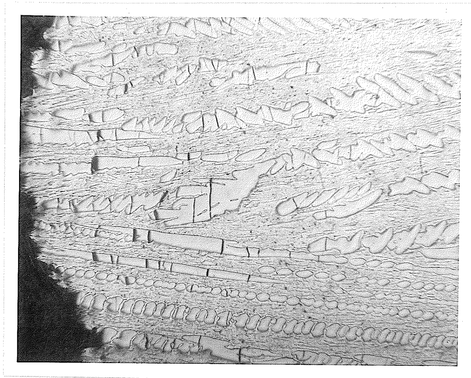
Fig. 48 Al-20%Ni fracture surface X 85
