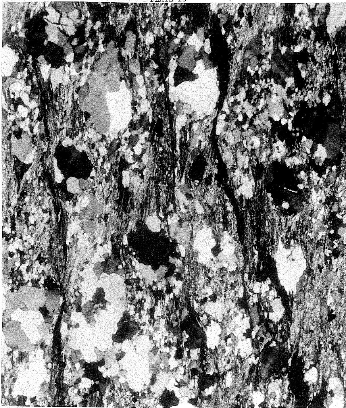
Photomicrograph of a sheared granodiorite now classified as a blastomylonite (X40, X-nicols). Absence of strain shadows may indicate complete recrystallization of quartz. Foliation direction is N 65°E.
