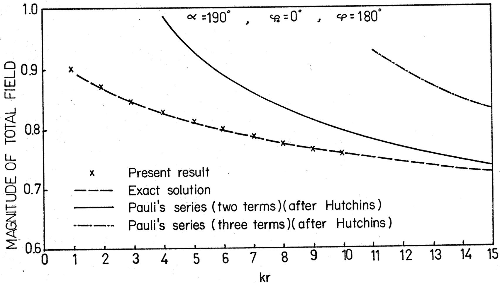
Fig. 2.2. Magnitude of the total field vs.  $kr$  for an H-polarized plane wave diffracted by a wedge (comparison between Pauli's series and the exact solution).
