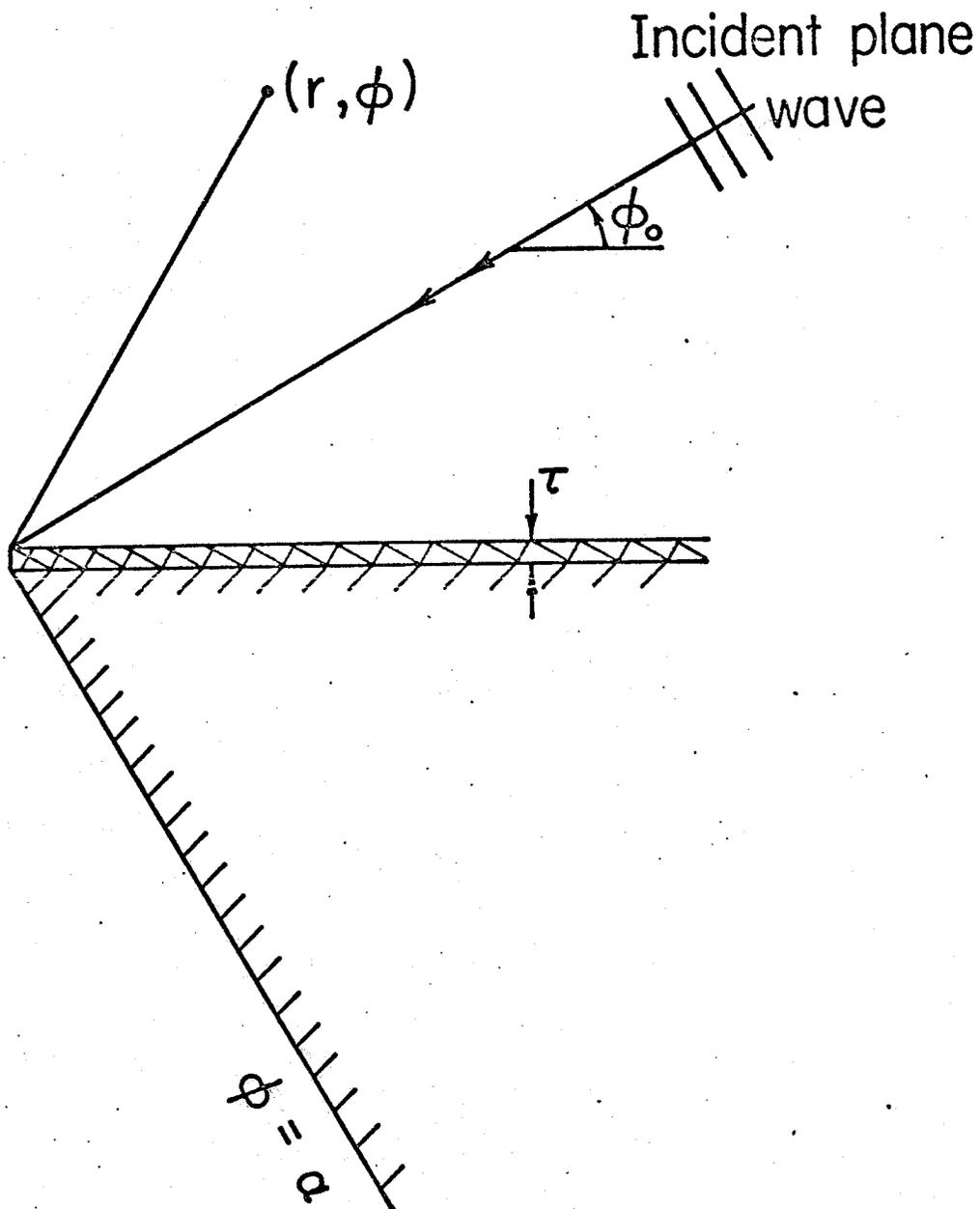
Fig. 3.1. Schematic diagram of a plane wave incident on a dielectric-loaded conducting wedge.
