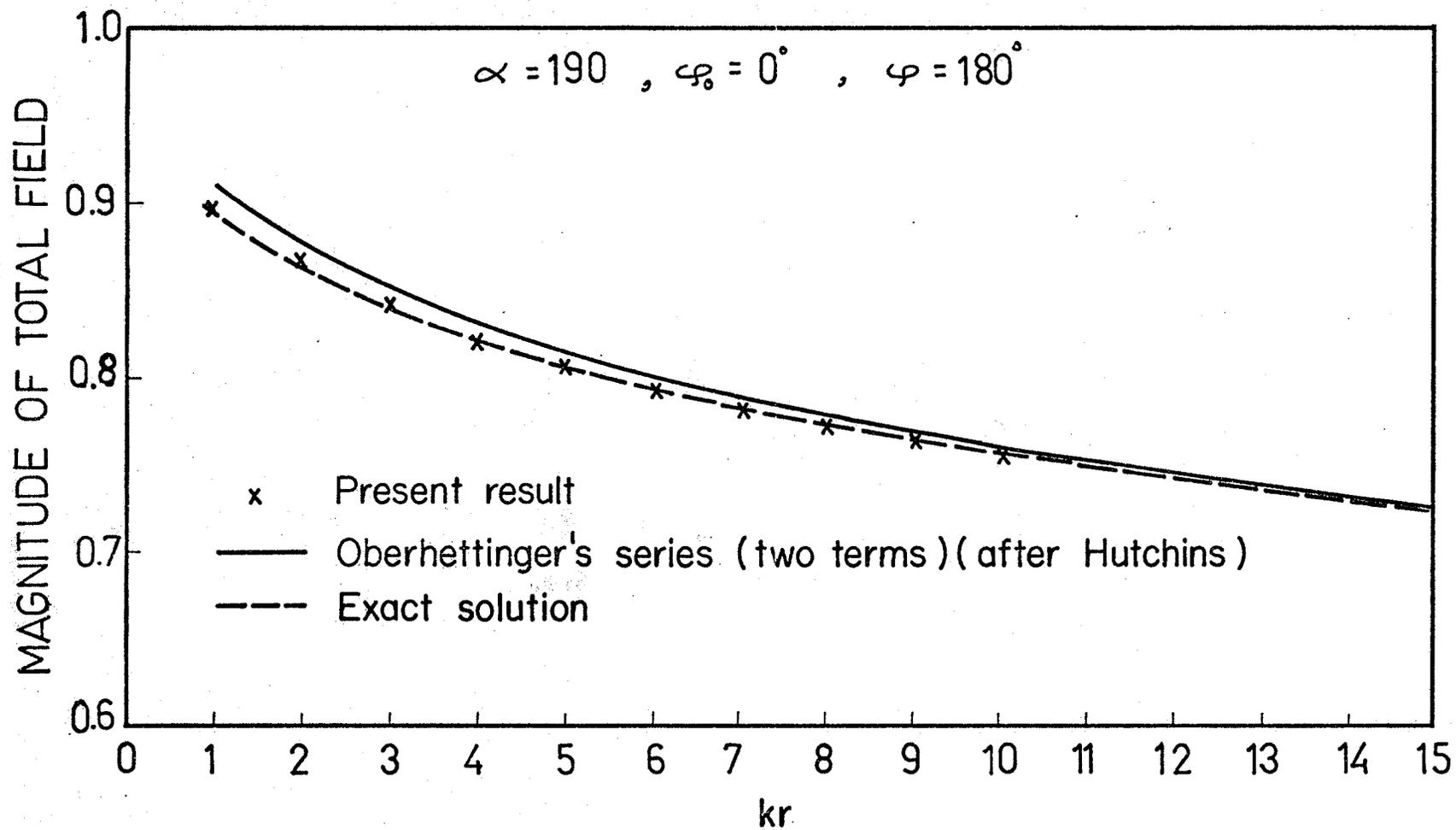
Fig. 2.4. Magnitude of the total field vs.  $kr$  for an H-polarized plane wave diffracted by a wedge (comparison between Oberhettinger's series and the exact solution).
