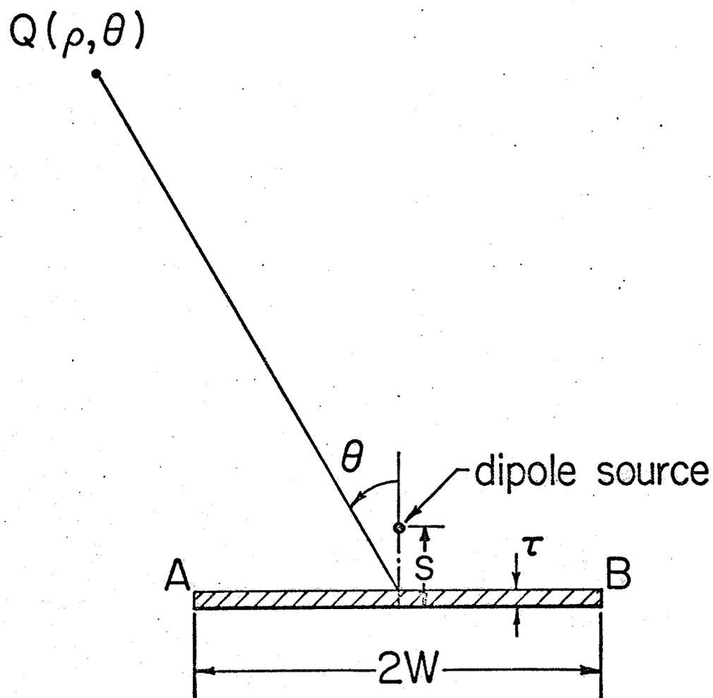
Fig. 4.1. Schematic diagram of a dielectric-loaded conducting strip fed by a dipole source.
