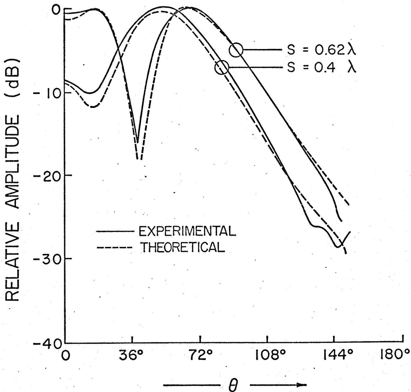
Fig. 4.5. Radiation pattern of the loaded strip ( $\tau = 0.127\lambda$ ).
