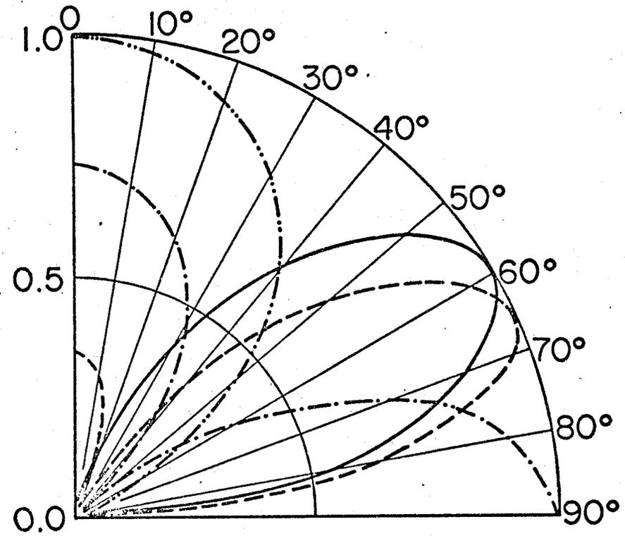
Fig. 5.1. Radiation pattern of a dielectric-loaded conducting plane.
