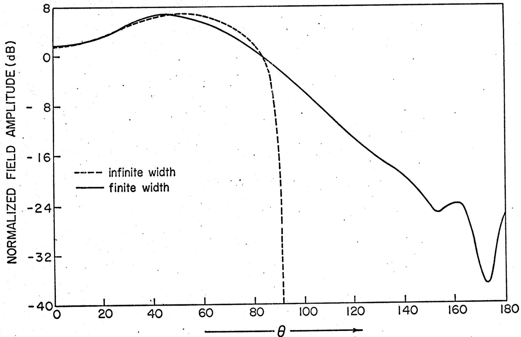
Fig. 5.2. Comparison between the radiation patterns of infinite and finite width ( $W = 1.4\lambda$ ) unloaded strip ( $s = 0.4\lambda$ ).
