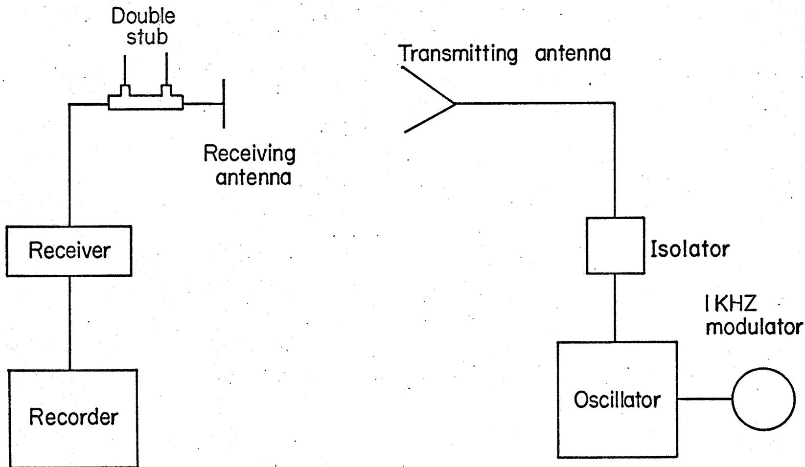
Fig. 4.3. Experimental set-up for measuring the radiation pattern of a dielectric-loaded strip.
