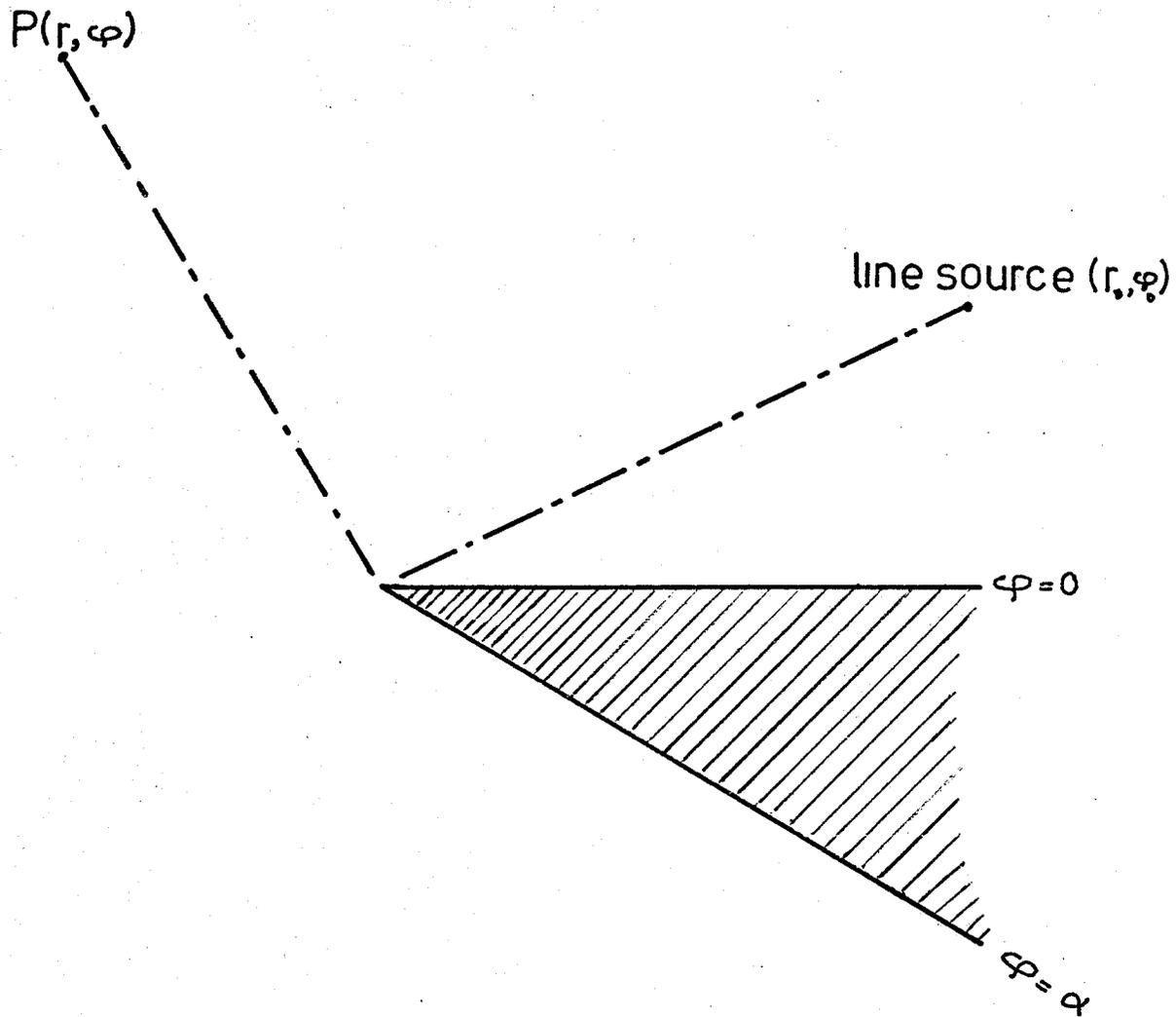
Fig. 2.1. Schematic diagram of a perfectly conducting wedge with line source excitation.
