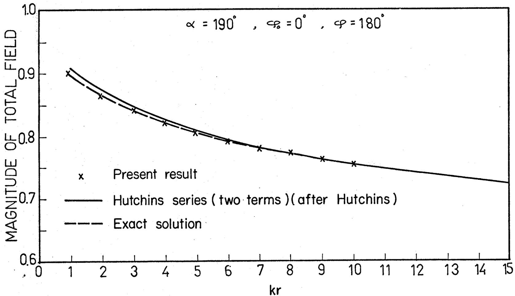
Fig. 2.3. Magnitude of the total field vs.  $kr$  for an H-polarized plane wave diffracted by a wedge (comparison between Hutchins' series and the exact solution).
