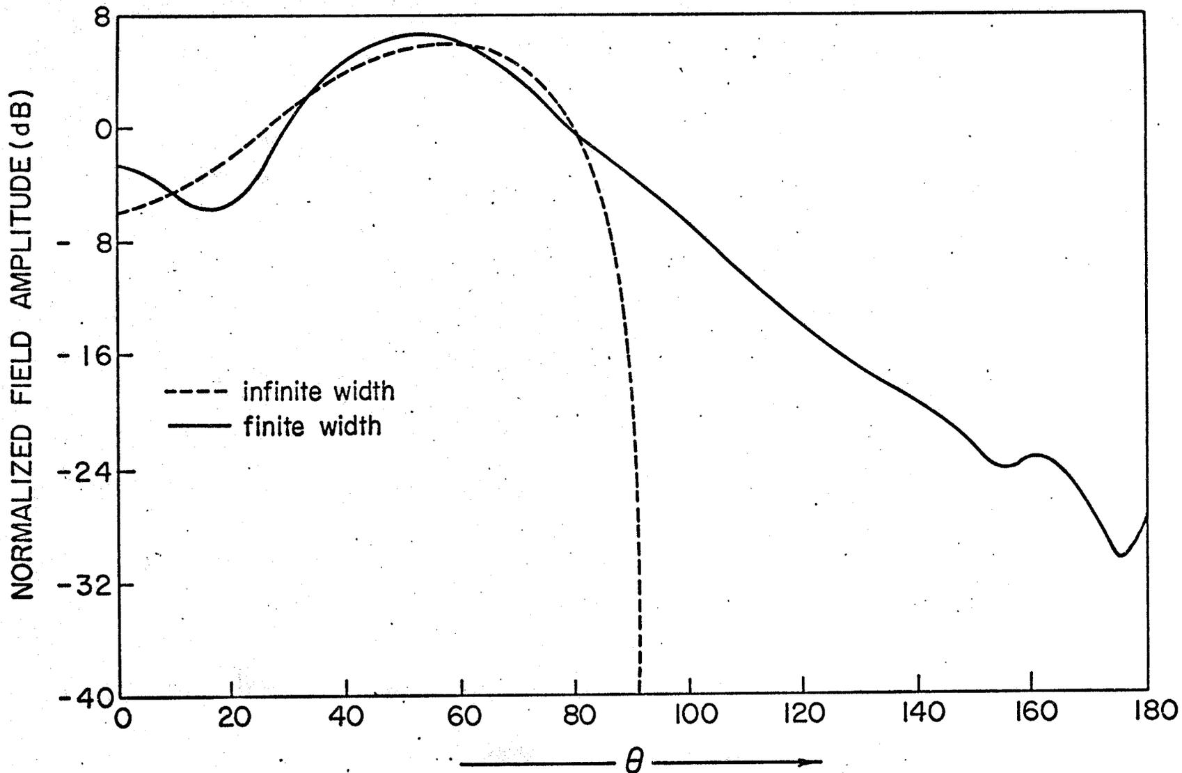
Fig. 5.3. Comparison between the radiation patterns of infinite and finite width ( $W = 1.4\lambda$ ) loaded strip ( $s = 0.4\lambda$ ,  $\tau = 0.127\lambda$ ,  $\epsilon_r = 2.59$ ).
