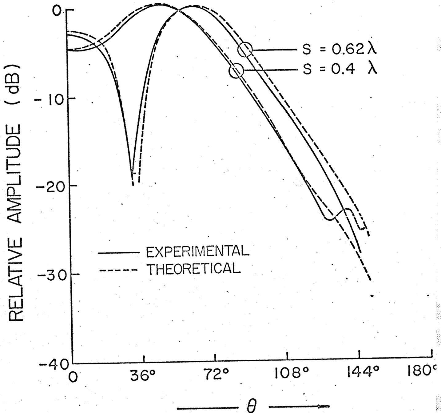
Fig. 4.4. Radiation pattern of the unloaded strip.
