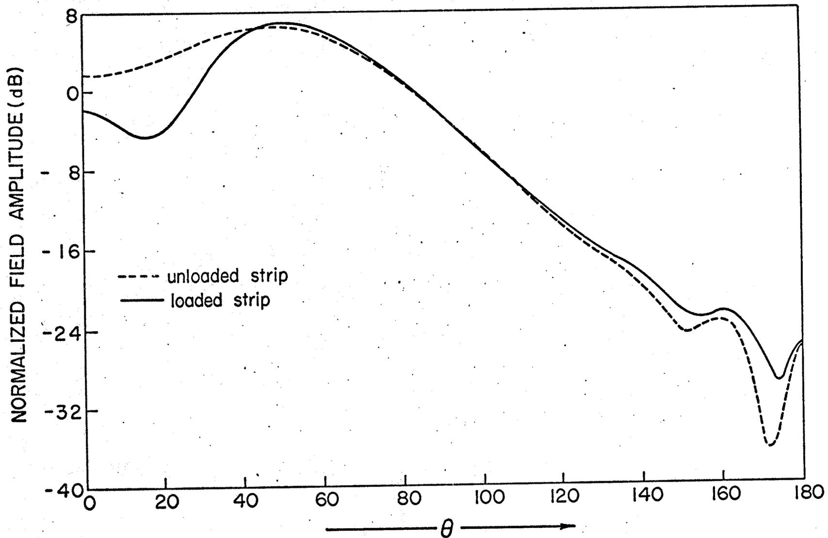
Fig. 5.4. Effect of dielectric loading on the radiation pattern of the strip ( $s = 0.4\lambda$ ,  $\tau = 0.127\lambda$ ,  $\epsilon_r = 2.59$ ).
