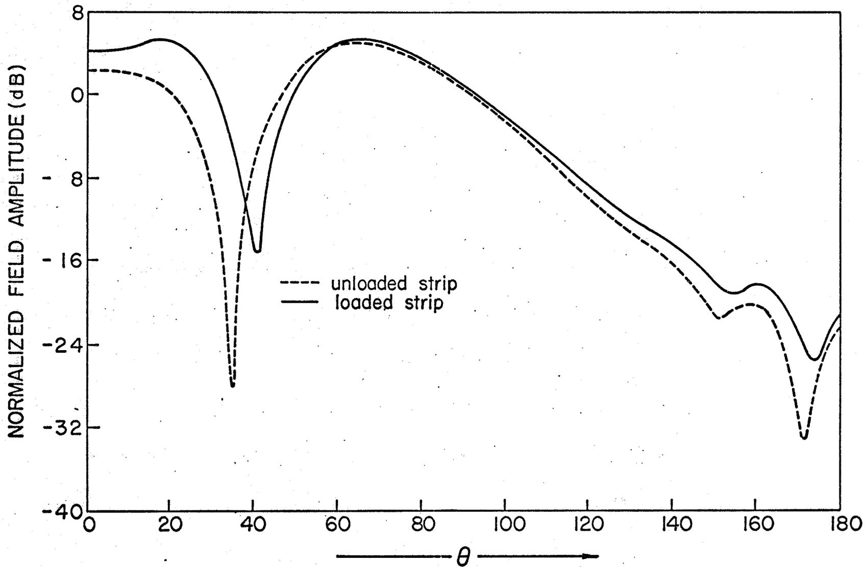
Fig. 5.5. Effect of dielectric loading on the radiation pattern of the strip ( $s = 0.62\lambda$ ,  $\tau = 0.127\lambda$ ,  $\epsilon_r = 2.59$ ).
