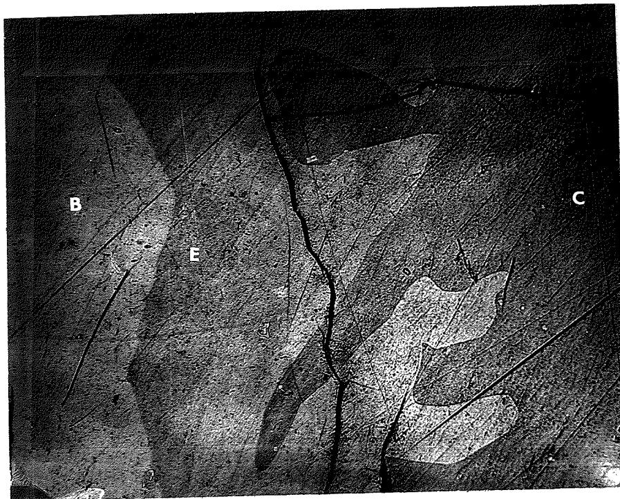
Figure 17c. \epsilon and \epsilon+\gamma region, heat treated Al-Mg couple, etched 5 secs. in 20% \text{HNO}_3 , B = \beta , E = \epsilon , C = \gamma , region between E and C is \epsilon+\gamma , 350x
