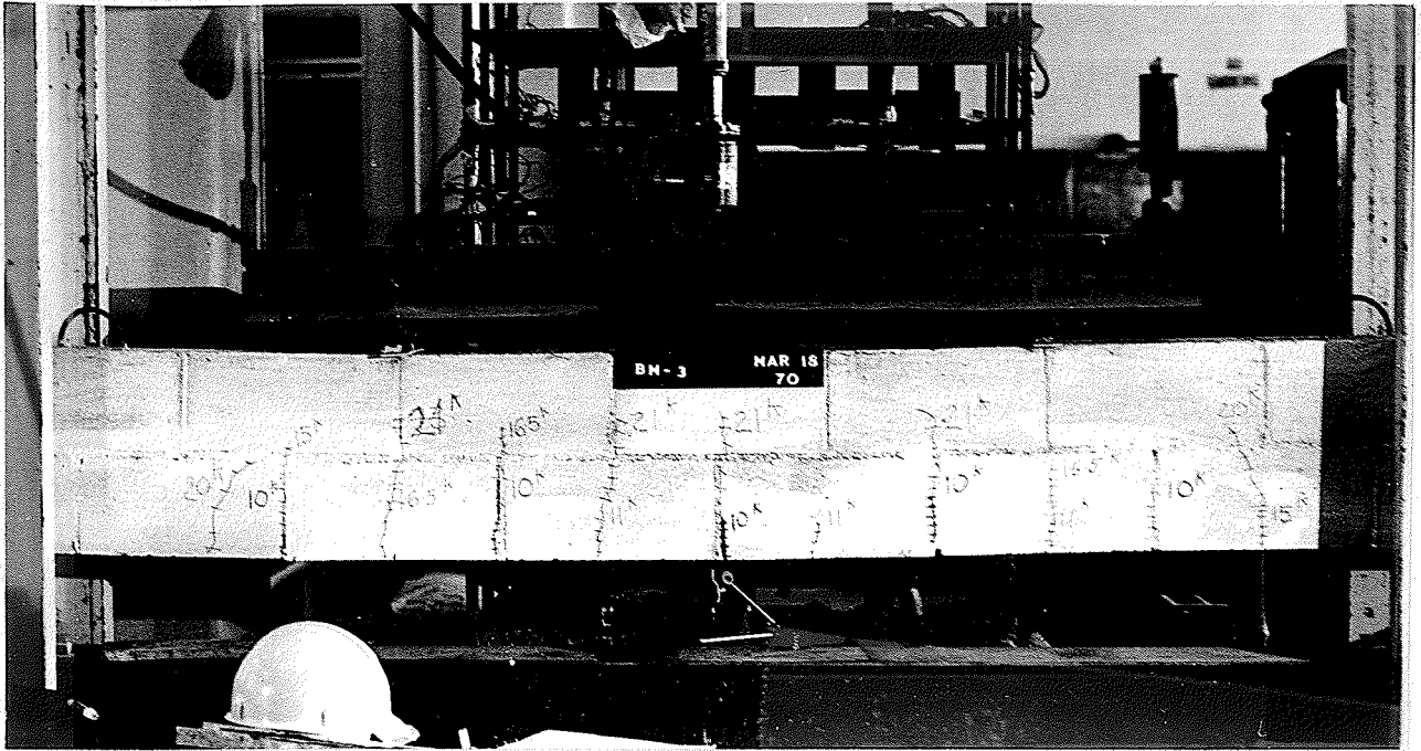
BEAM 3 SHOWING FLEXURAL FAILURE FIGURE 39
