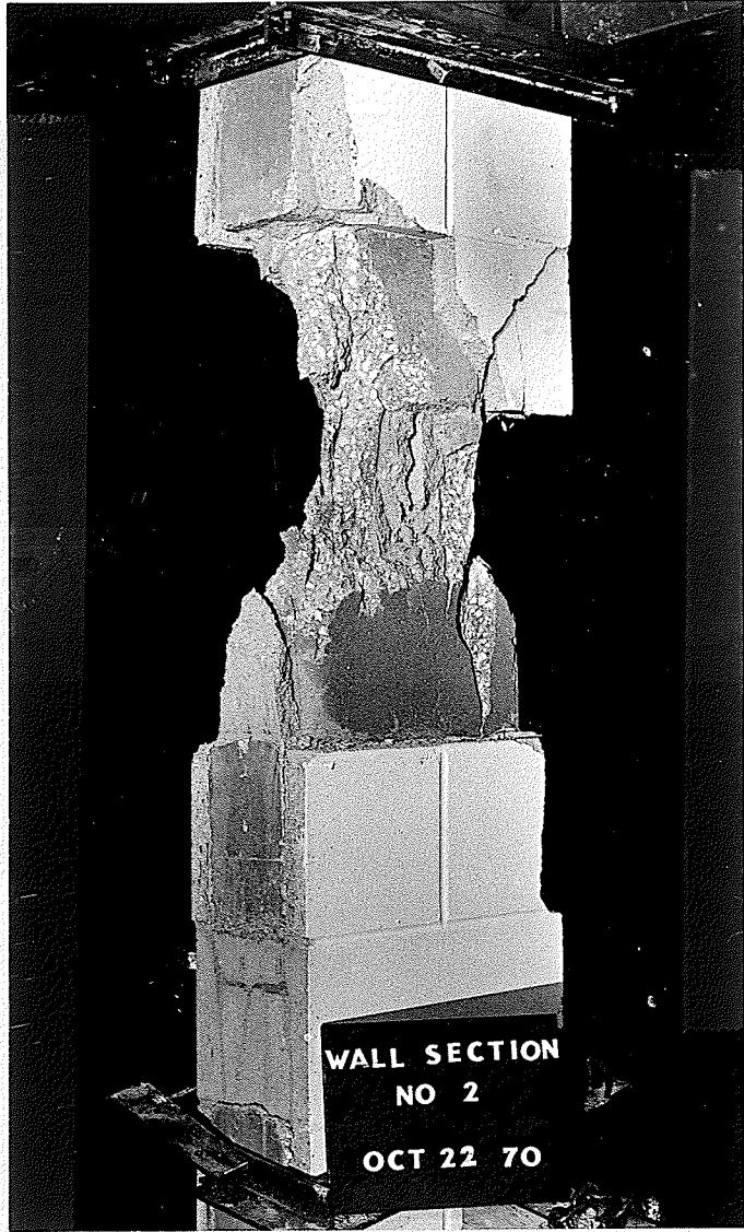
WALL SECTION 2 AT FAILURE
