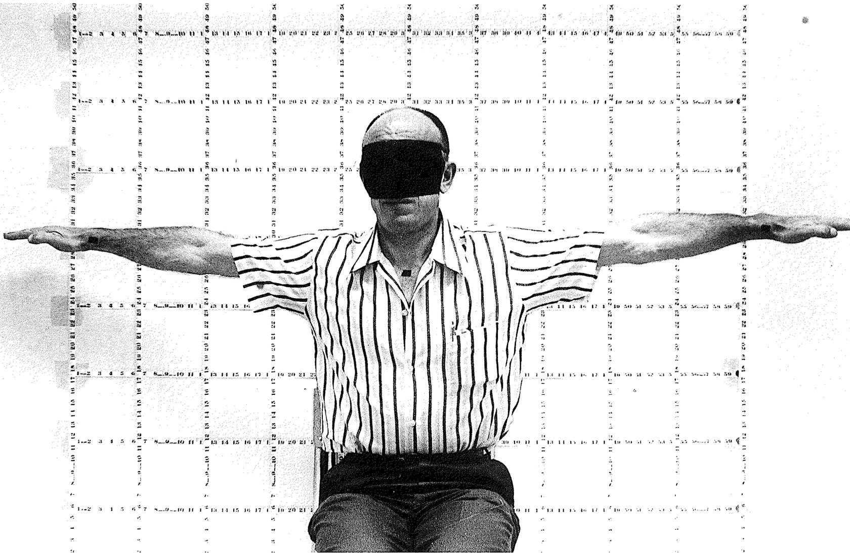
tape 1 in. wide was fixated around the midpoint of the dowel. Stripes of black electrician's tape approximately .5 in. long was placed on each S's wrist, the tip of the middle fingers, and at the neck. These strips of tape were used to facilitate the measurement of the different postural positions. After photographing the S's in front of the grid, the strips appeared as points representing coordinates on a Cartesian graph.
