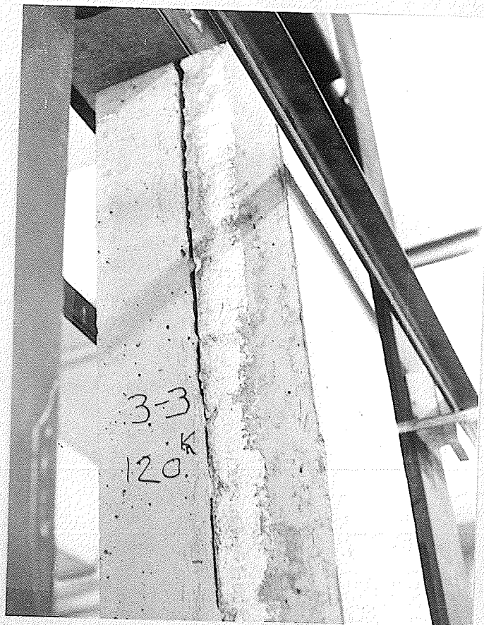
Plate No. 28. Showing panel 3 - 3 during test.
