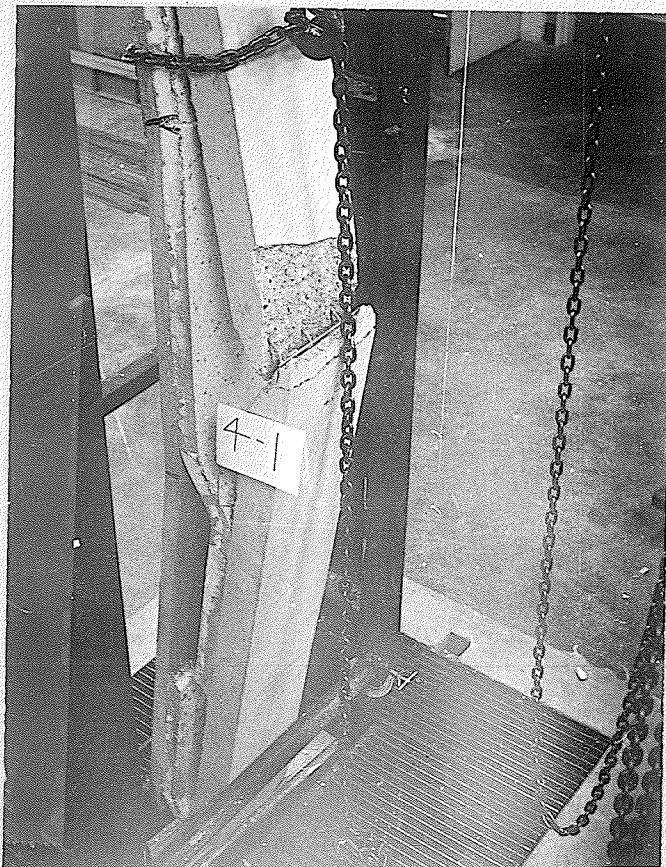
Plate No. 20. Showing panel 4 - 1 at failure.
