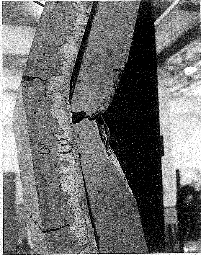
Plate No. 29. Showing panel 3 - 3 at failure.
