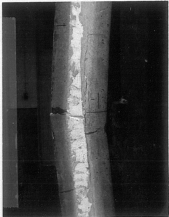
Plate No. 30. Showing panel 1 - 1 at failure.
