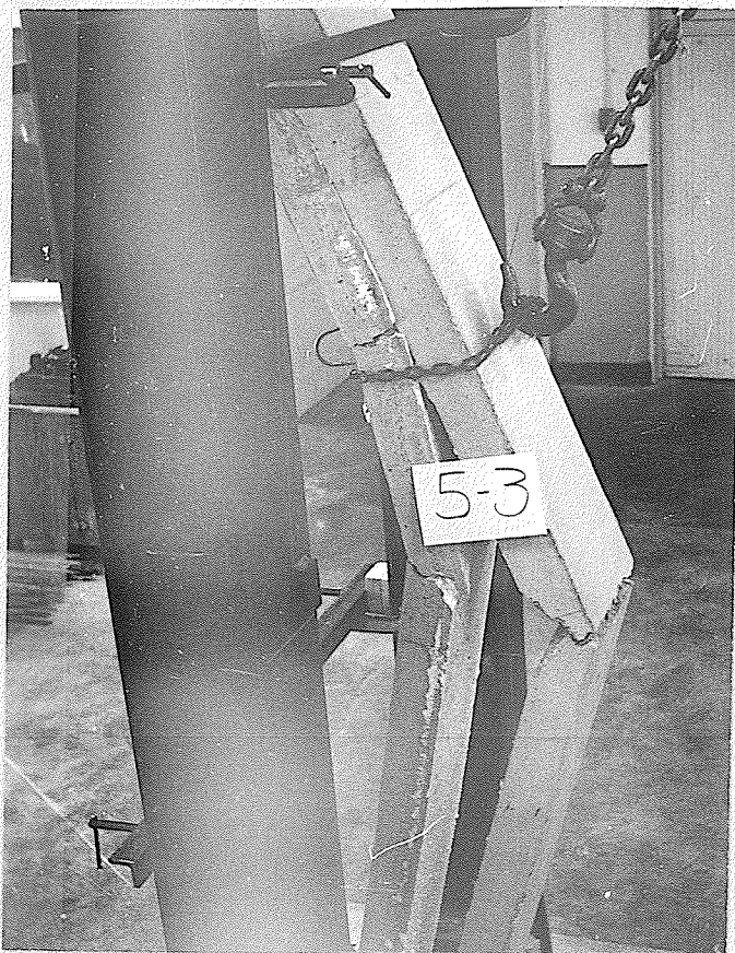
Plate No. 16. Showing panel 5 - 3 at failure.
