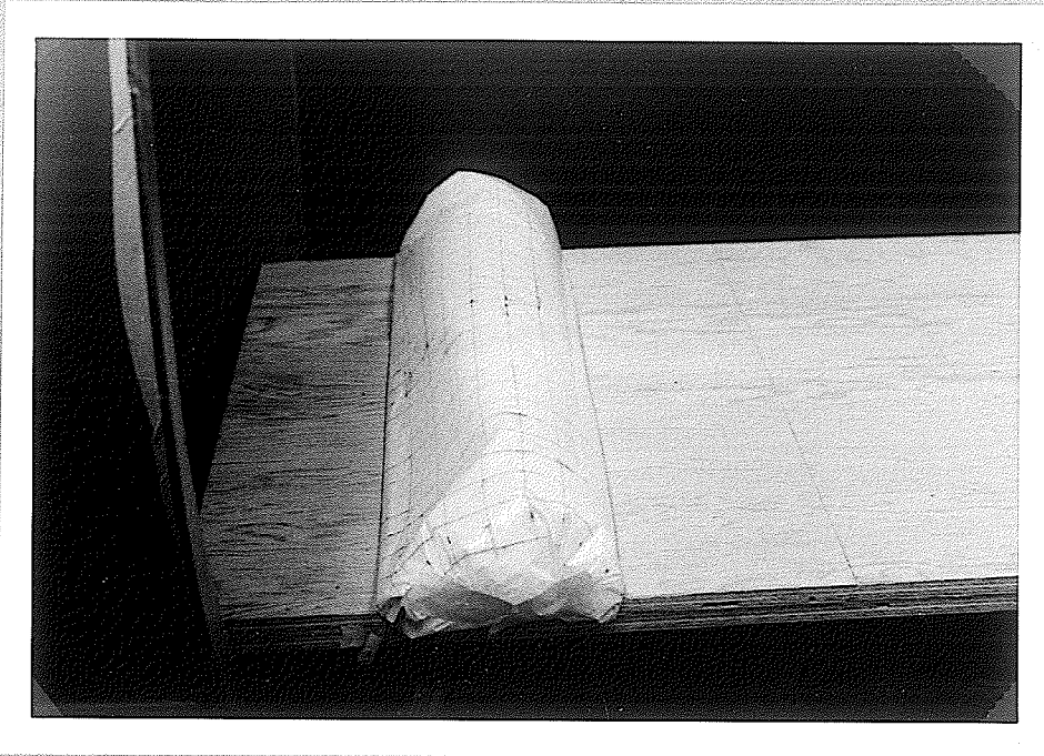
Fig. 22 Inflation of membrane with wind blowing stage 2 almost full
