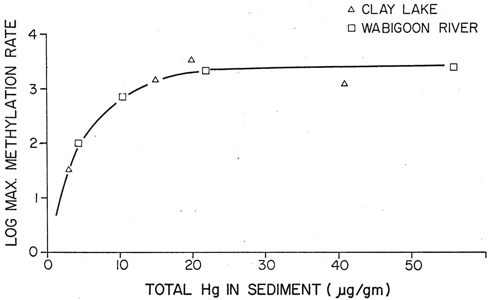
Figure 17. Log level-off rate of net methyl mercury release (level-off values taken from Figs. 8 and 9) from Clay Lake and Wabigoon River microbasins as a function of total sediment mercury concentration.
