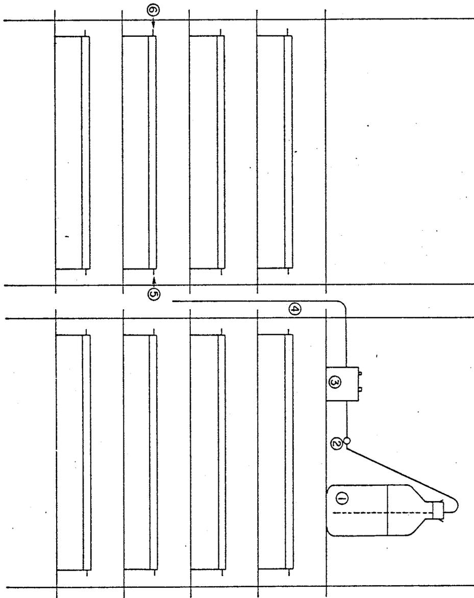
mercury content which was indicative of the net methyl mercury release from the sediments within the basin. Effluent from each microbasin was collected in a 1<sup>l</sup> bottle so that the amount of water flowing through the basin could be monitored daily; Volumetric flasks (1<sup>l</sup> ) were utilized to collect effluent, over 24 hours, for analysis. The loss of methyl mercury from the volumetric flasks over the 24 hour collection period was found to be < 10%.
