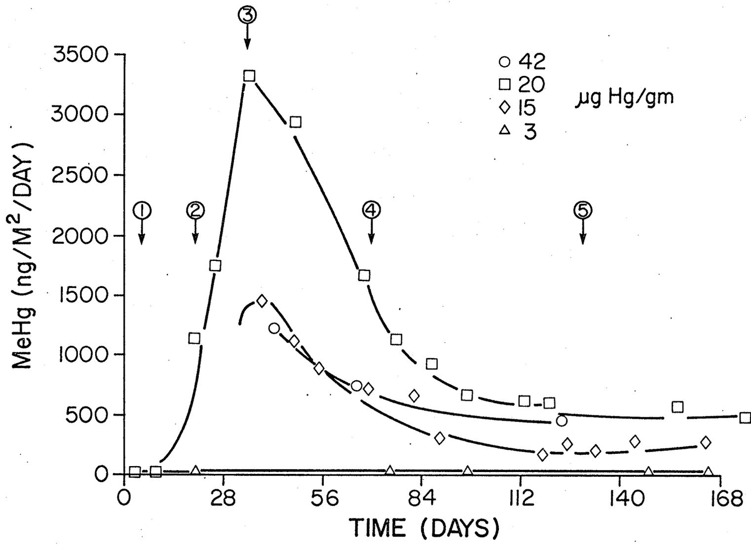
Figure 9. Net release of methyl mercury from mercury contaminated Wabigoon River sediments as a function of time. Characteristics (i.e. lag, etc.) same as in Fig. 8.
