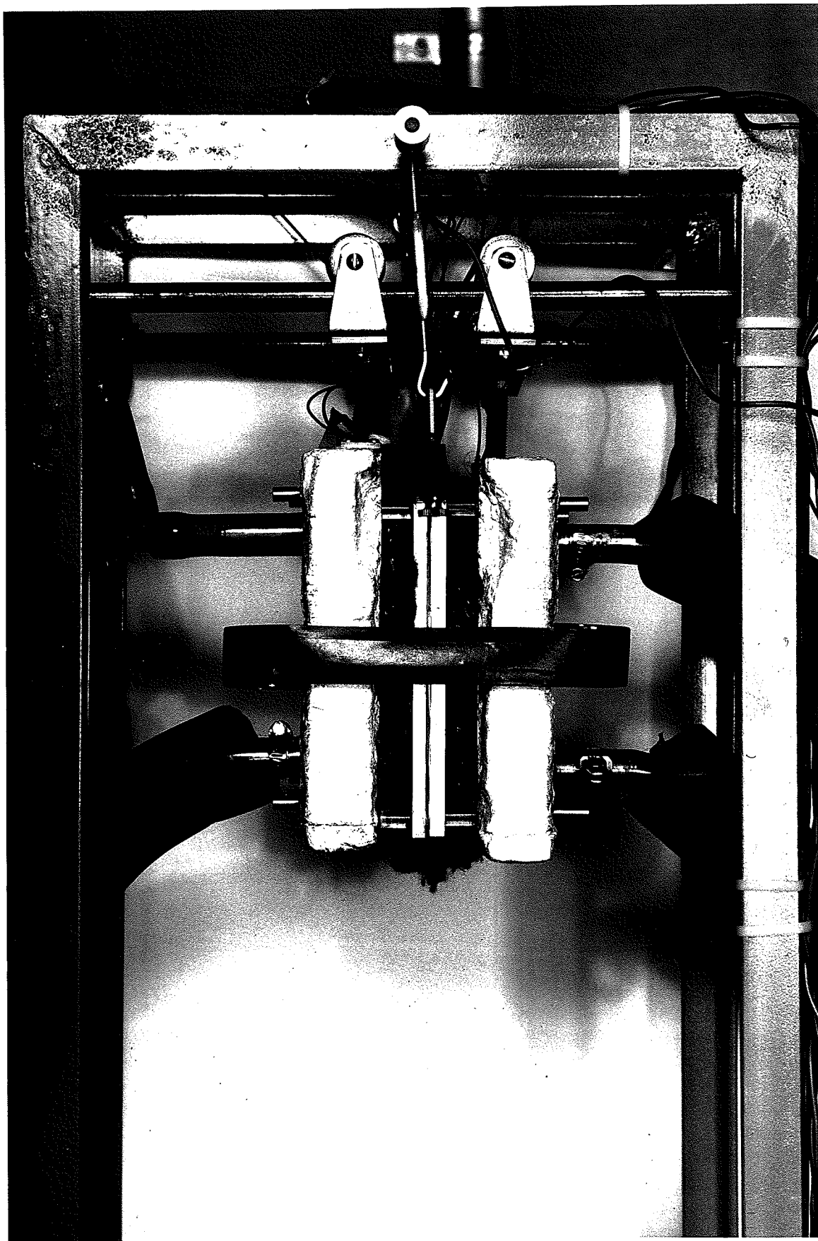
Plate 3. Plate Assembly with Three-Layer Multifiber Batt-Assembly, Plexiglas Spacers, and Coil Spring in Place.
