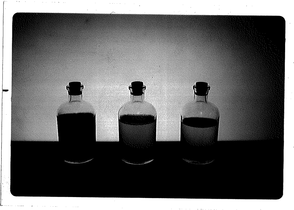
Figure 4.6.1. Samples of diluted swine manure slurry subjected to ozonation for 0, 5, and 10 h (l to r).
