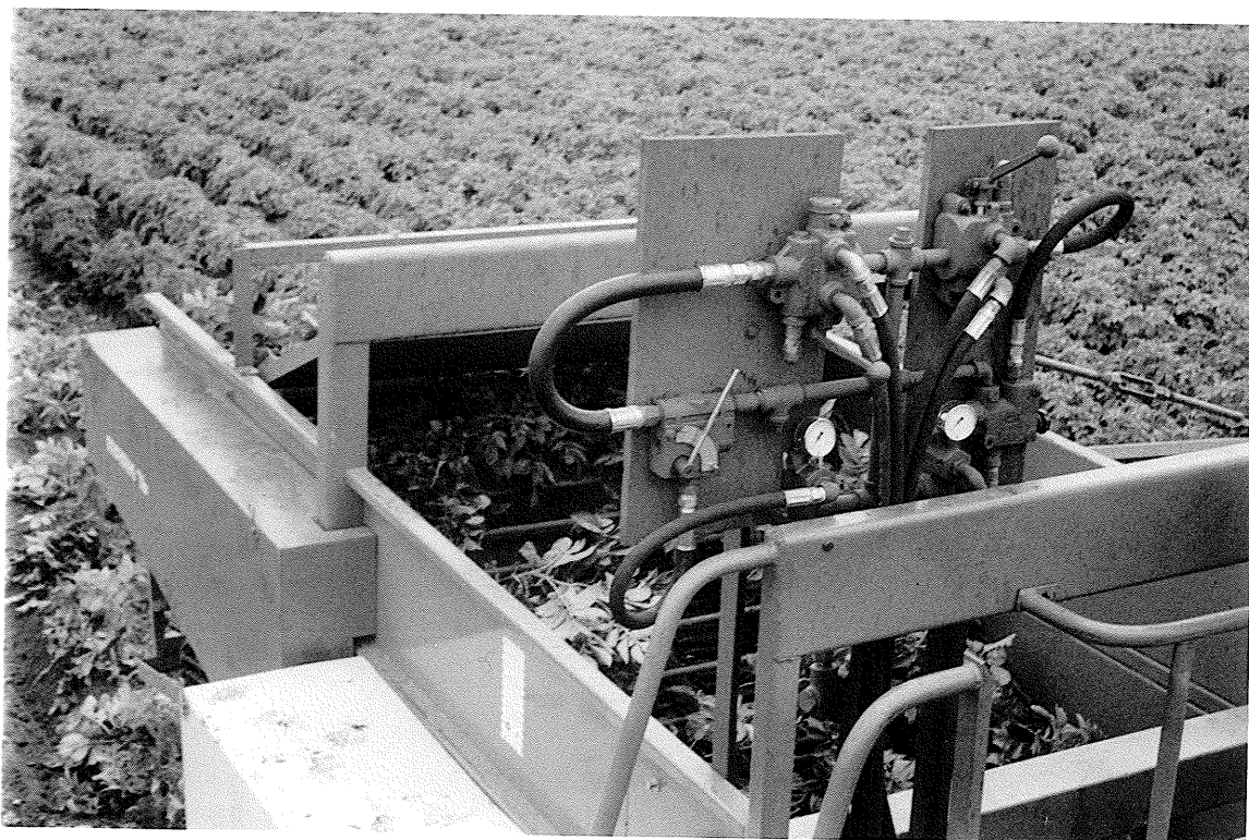
Fig. 3.6 View of Control Panel Illustrating the Flow Control Valves and Accessories.
