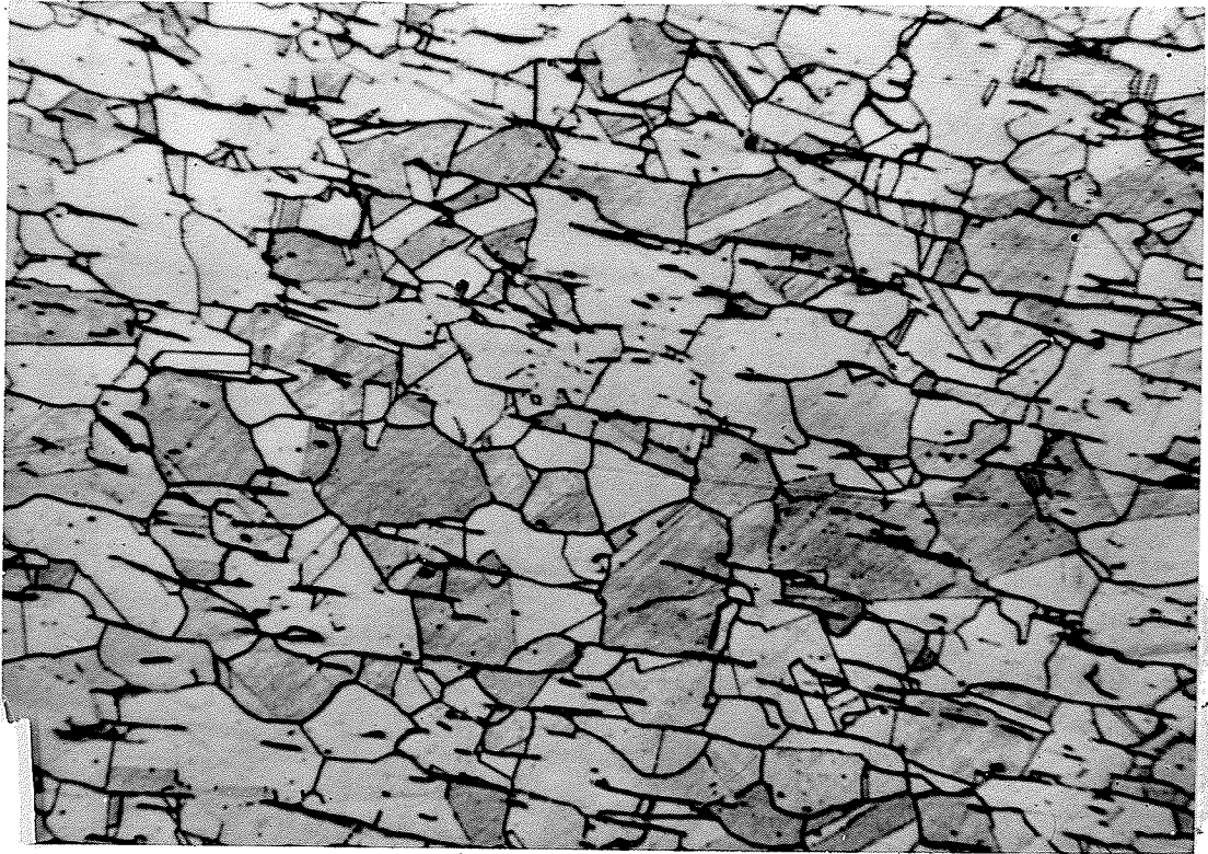
Fig. 15 Appearance of aligned precipitation phase bears resemblance to inclusions. Precipitate was formed during forging before final stress-relief anneal as they can be seen to extend into the recrystallized grains. Etched electrolytically in 10% oxalic acid (180x)
