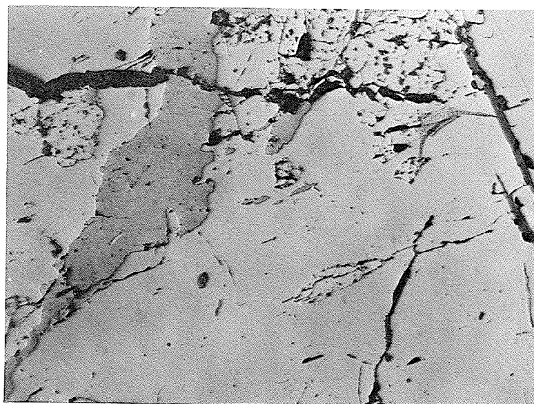
Plate XXI Chalcopyrite-pyrrhotite. Elongate chalcopyrite grain cutting across pyrrhotite. Small blebs to the right of the chalcopyrite grain in the central part of the photo are chalcopyrite exsolution blades in pyrrhotite. Plane light, X31. (1002)
