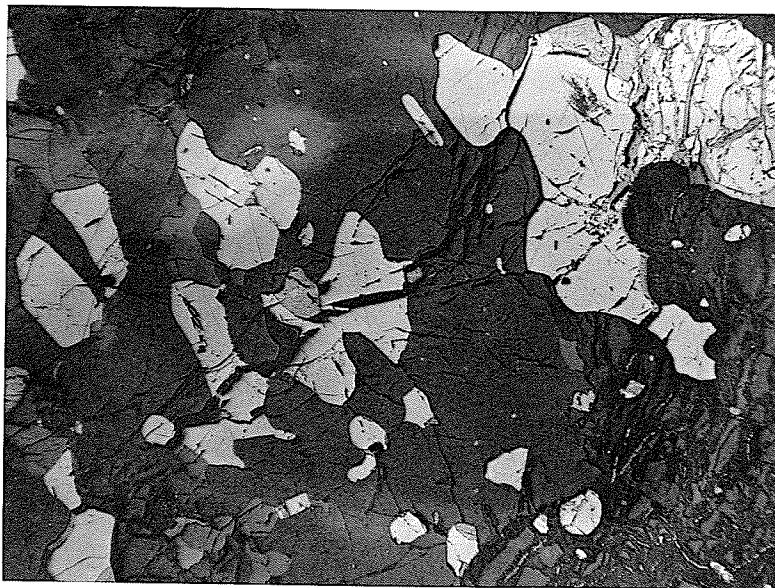
Plate IX Chromite-sulphide relationships. Sulphide blebs and wholly enclosed by individual chromite grain (lower central). Remainder of sulphide is interstitial. Plane light, X31. (602).
