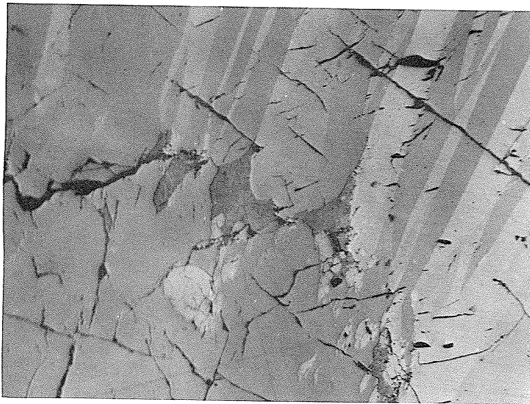
Plate XVI Twinned pyrrhotite. Note delicate exsolution flames of pentlandite associated with terminations of pyrrhotite lamellae. Crossed nicols, X36, (739)
