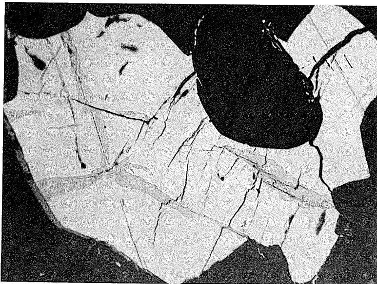
Plate XI Cubanite exsolution blades in chalcopyrite. Note three directions of orientation of blades, and interstitial nature of chalcopyrite. Crossed nicols, X122. (536).
