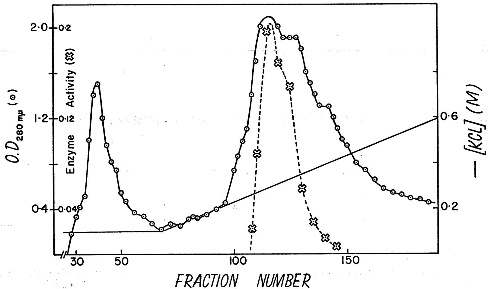
FIGURE 2. Elution of PEP carboxylase from G-150 Sephadex column. Optical density was measured at 280 m $\mu$  and enzyme activity in the fractions was measured spectrophotometrically as described in "Methods". Three ml fractions were collected at 4 $^{\circ}$ .
