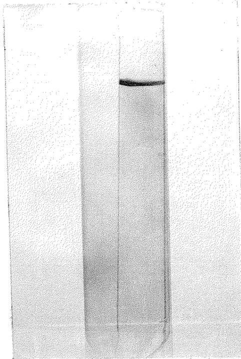
Appearance of PEP carboxylase in polyacrylamide gels after electrophoresis and staining with Coomassie blue ("Methods"). Approximately 50  $\mu$ g of the enzyme was applied to the gel.
