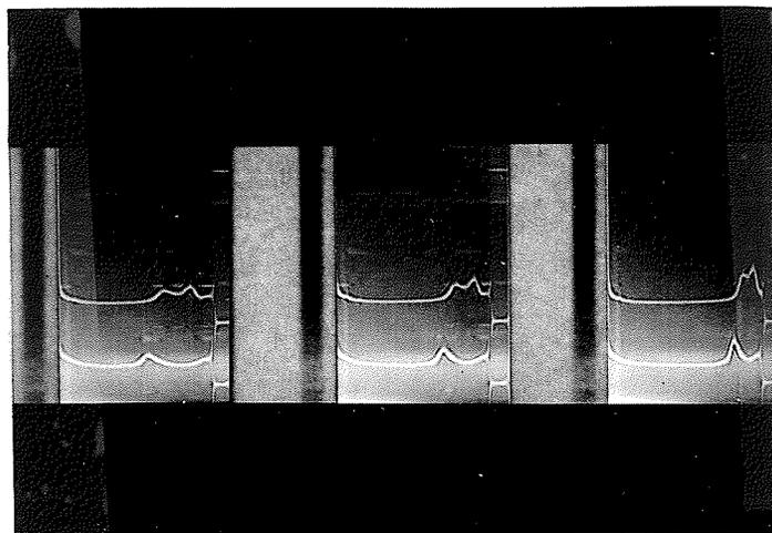
Schlieren pattern of PEP carboxylase during sedimentation velocity runs with Model E ultracentrifuge ("Methods"). The upper curve shows dissociation of the enzyme after storage of enzyme in 0.05 M Tris-HCl (pH 8.0) for 20 hours and the lower curve shows the re-association in the presence of 50 mM mercaptoethanol. Pictures were taken at 8, 16 and 24 minutes (left to right) after rotor had reached 44,000 rpm.
