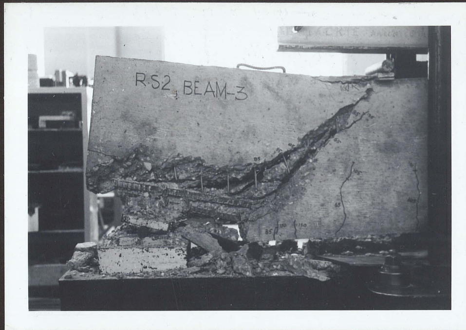
FIG. 54 - Beam 3: View on side R.S.2 after Complete Failure
