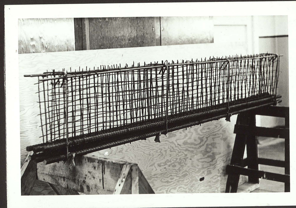
FIG. 22 - Side View of Reinforcement cage for Beam 6
