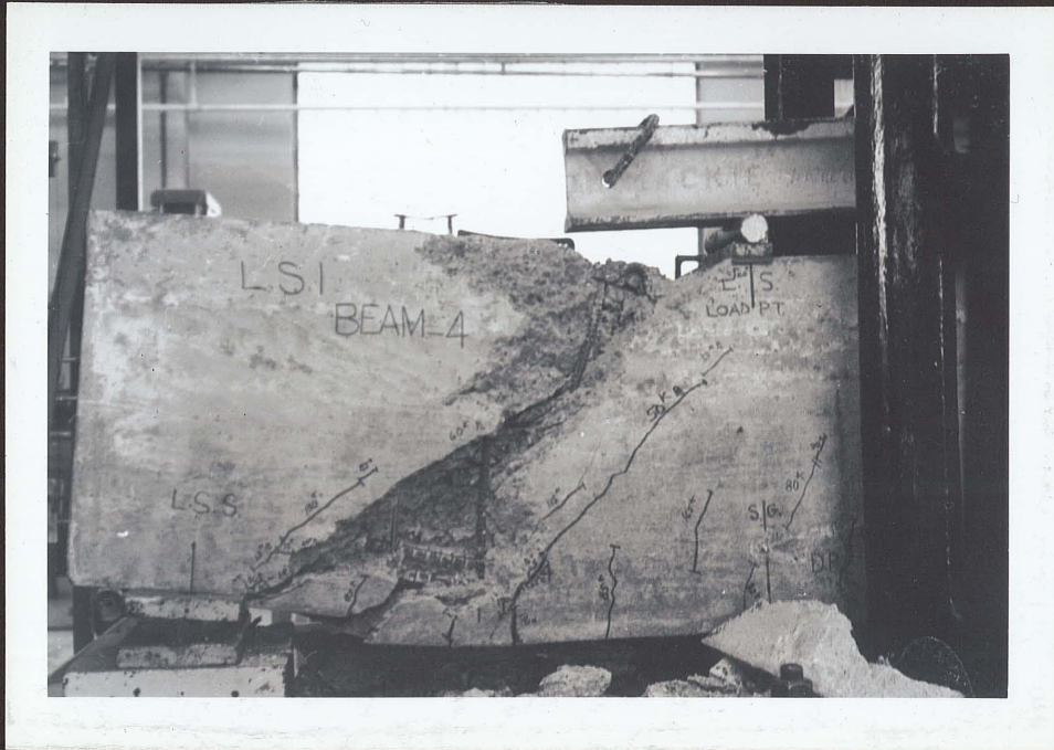
FIG. 58 - Beam 4 (side L.S.1) on Further Loading after Failure
