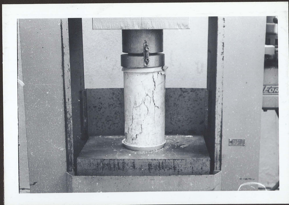
FIG. 36 - Compression Failure of the Cylinder
