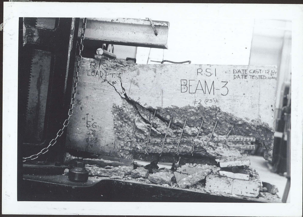
FIG. 53 - Beam 3 on Further Loading after Failure
