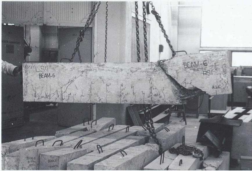
FIG. 68 - Beam 6 after Failure (side L.S.1 - R.S.1)
