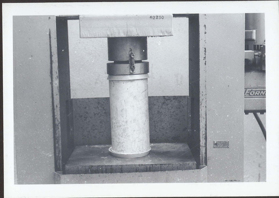
FIG. 35 - Test Cylinder before Application of the Load
