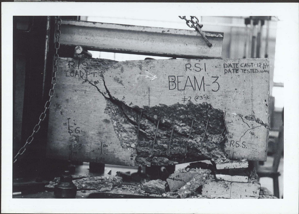
FIG. 52 - Beam 3 after Failure (side R.S.1)
