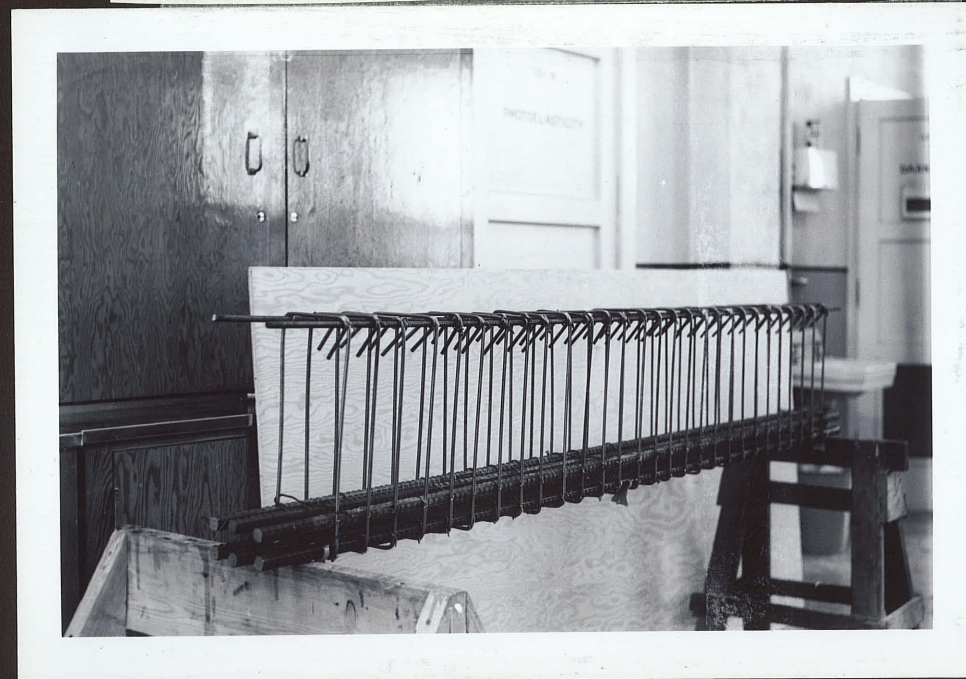
FIG. 17 - Reinforcement Cage for Beam 3
