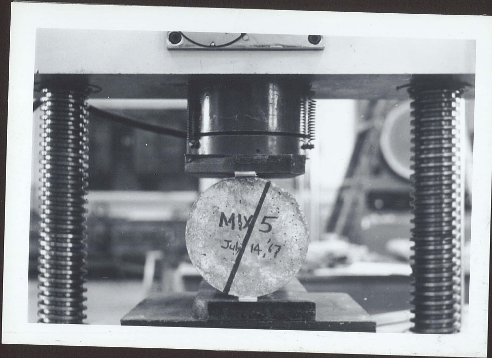
FIG. 37 - Arrangement for Tensile Splitting Test
