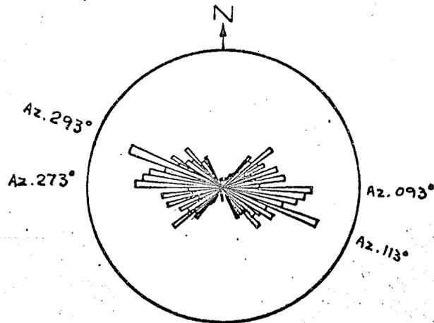
SYNOPTIC ROSETTE DIAGRAM, SUMMARIZING THE STRIKE READINGS OF 695 UNITS OF THE FIRST ORDER LINEAMENTS. RADIUS OF THE CIRCLE REPRESENTS TEN PERCENT OF THE TOTAL NUMBER OF FIRST ORDER LINEAMENTS.
