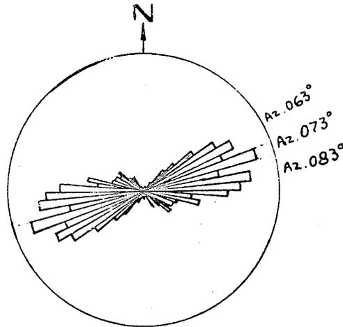
SYNOPTIC ROSETTE DIAGRAM, SUMMARIZING THE STRIKE READINGS OF 1,859 SECOND ORDER LINEAMENTS. RADIUS OF THE CIRCLE REPRESENTS TEN PERCENT OF THE TOTAL NUMBER OF SECOND ORDER LINEAMENTS.
