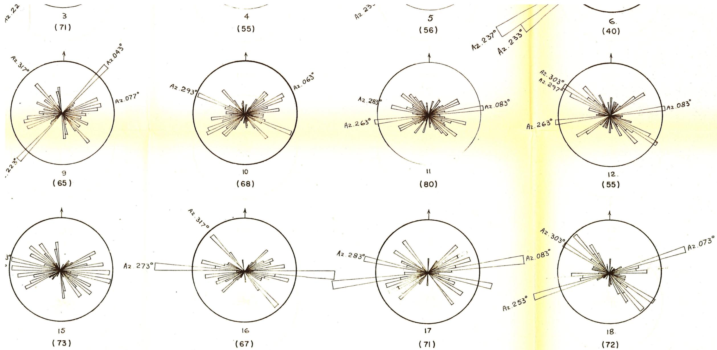
DIAGRAMS OF FIRST ORDER LINEAMENTS FOR EACH SUBAREA. RADIUS OF EACH SEGMENT REPRESENTS TEN PERCENT OF THE TOTAL NUMBER OF FIRST ORDER LINEAMENTS IN THAT SUBAREA. SEGMENTS ARE DIVIDED INTO 5-DEGREE SEGMENTS.
