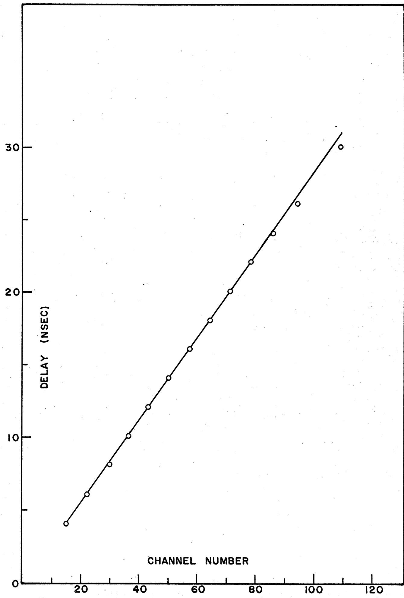
longer operating in its linear region. This could be improved by adjusting the circuit parameters but only a 20 nanosecond range is required in actual operation. This calibration curve does not exhibit the slightly sinusoidal shape caused by the ringing of the limiter pulses indicating that the damping resistor reduced or eliminated this fault.
