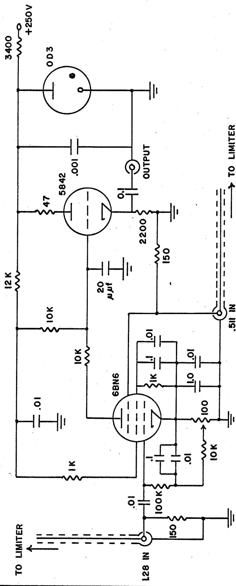
grids to which the limited pulses are applied. A significant plate current will flow only if both grids are driven positive simultaneously. Therefore, the tube conducts only when the limited pulses to the control grids overlap. The time during which conduction occurs (the length of the anode pulse) is determined by the amount of overlap. The length of the anode pulse is then converted to a pulse height by a standard integrating circuit employing a 5842 triode.
