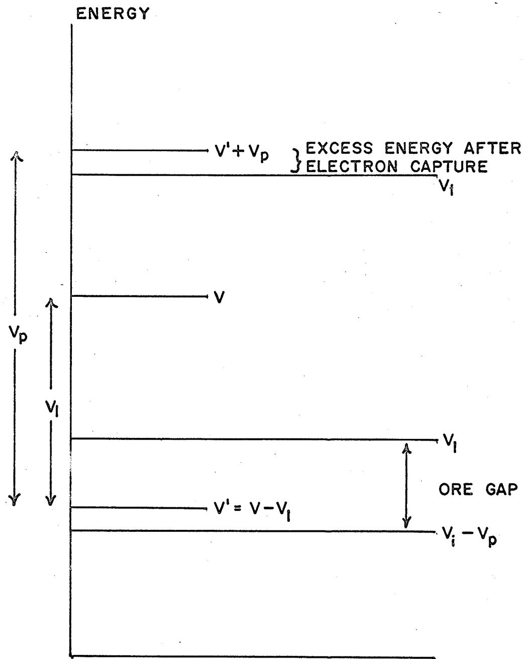
of positronium since, according to the Ore model, positrons which have passed through the Ore gap without forming positronium are recycled through it and given another opportunity to capture an electron.
