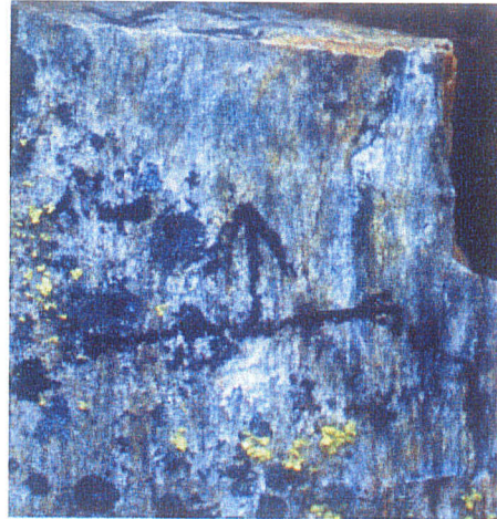
Figure 7.10 Highly siliceous pseudo mylonite to mylonite near Councill Lake. Includes 1-2% disseminated sulphide minerals and trace quantities of gold. Easting 367431, northing 6283210; UTM Zone 14, NAD83.
