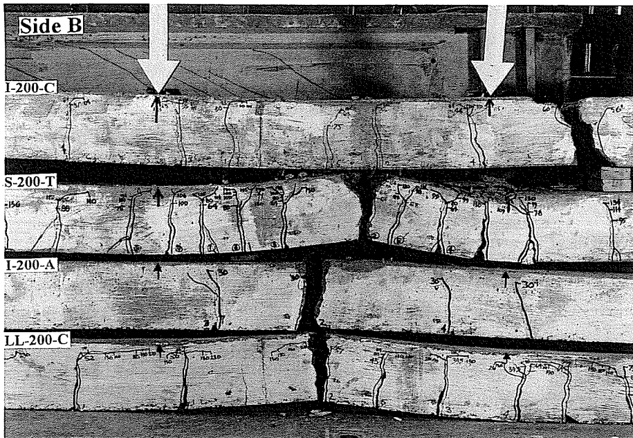
Figure 4.20: Crack patterns of the 200 mm thick slabs.
