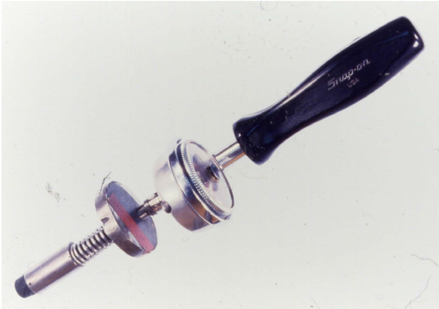
Figure 3.3. Modified torque wrench used to measure tuber skin-set (after Lulai and Orr, 1993).
