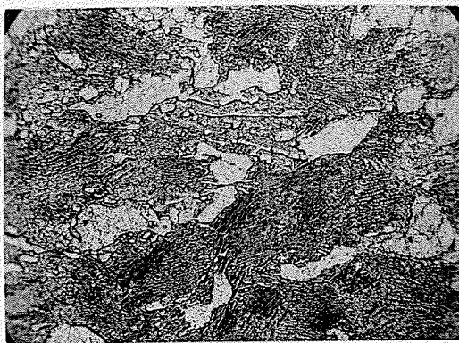
Plate 49. Alloy 39, X 250. As cast; \alpha -2 (light) in a eutectic matrix of \delta -1 and \alpha -2. Note difference (re plate 27) in appearance of lead crystals when indium is present.
