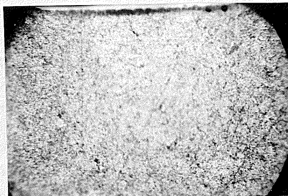
Plate 24. Alloy 12, X 250. No evidence present of heterogeneity of the sample; same appearance as alloy 11, plate 22.
