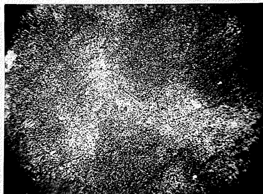
Plate 25. Alloy 12, X 135. Repolished and reetched after 3 months at room temperature; \alpha -2 (light) with \beta -2, heterogeneity now being evident.
