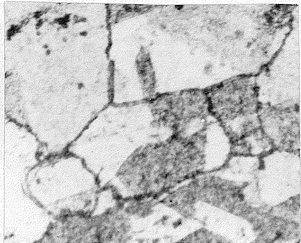
Plate 34. Alloy 25, X 1000. Upper center of plate 33, indicating that the dark spots are particles of \beta showing the pitted features met before for this phase.
