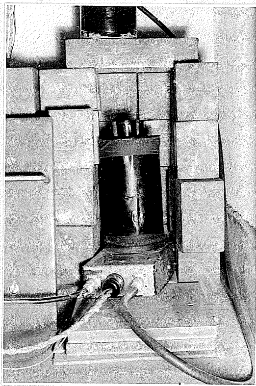
fig. 5d. Showing Photomultiplier Tube Housing and Cathode Follower in Lead Castle
