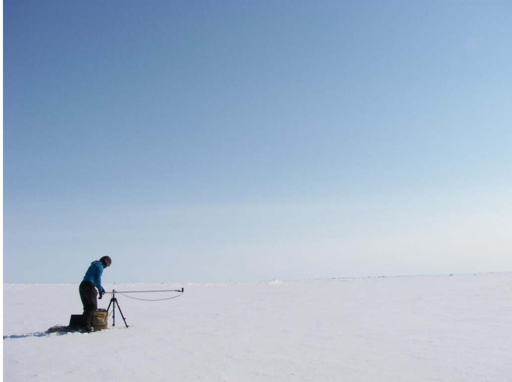
FIGURE 13. Setting up the spectroradiometer (ASD) to measure downwelling and upwelling radiation during the melting period.
