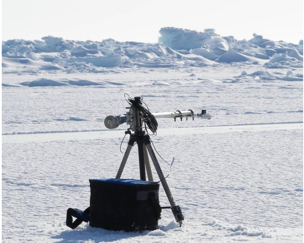
FIGURE 11. Licor PAR sensor set-up for albedo measurements.
