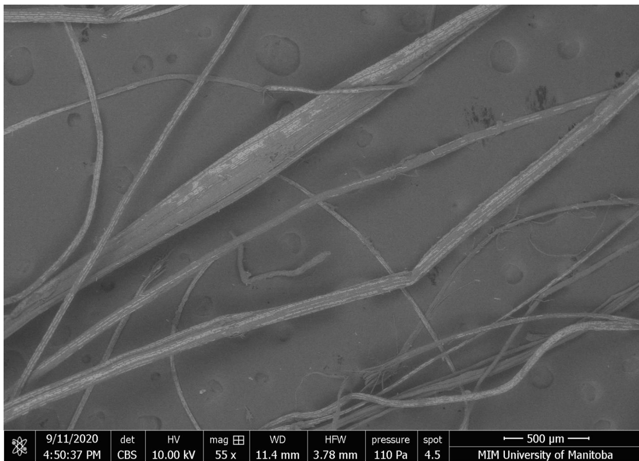
Figure 6.2.1.6. A backscattered electron image capturing the same place as Figure 6.2.1.5. Some fibers had calcium oxalate plates on their surfaces in this image.
