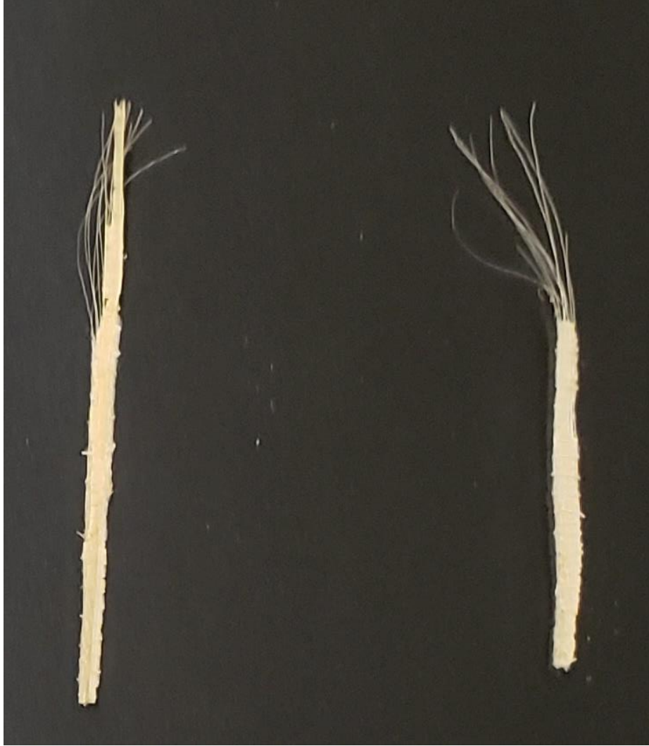
Figure 4.1.10. The column on the left contained partition materials, which caused a difficult extraction process; the column on the right did not contain or contained fewer partition materials and therefore an easier extraction process resulted.
