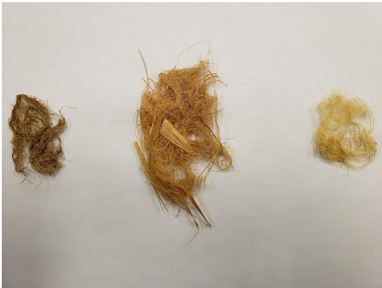
Figure 6.2.3.2. A photo showing fibers extracted from different parts of Typha leaves by chemical extraction. Left: fibers from lamina; middle: fibers from sheath; right: fibers from sheath with the ventral and dorsal surface removed. Different colors could be observed.
