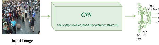
Figure 3.4: Local Scale Attention Network. This module produces three feature maps of size H/4 \times W/4 each of which associated to a density scale. C(i, j) denotes a 2D convolution with a filter size of i \times i and with j output feature maps. P stands for max pooling.
