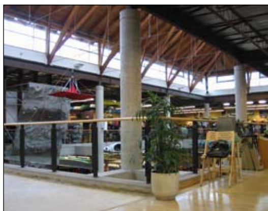
Figure 4.61 The upper level of the store is open to permit natural light from skylights to penetrate to the ground floor.
