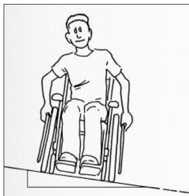
Figure A48: Off-balance pedestrian in wheelchair on a cross slope
