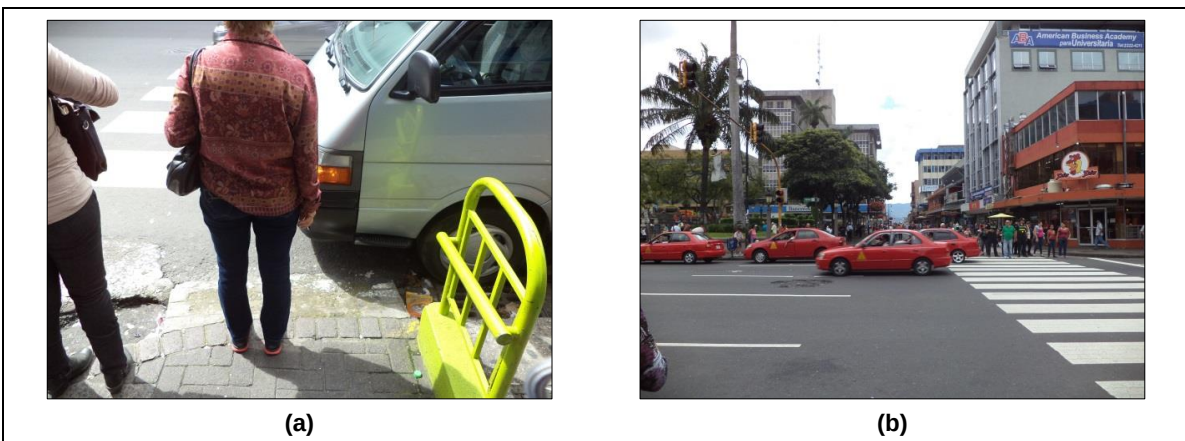
Figure 13: Activity in outer lanes blocks curb ramps at crosswalks: (a) Parked vehicle; (b) Taxi stand
