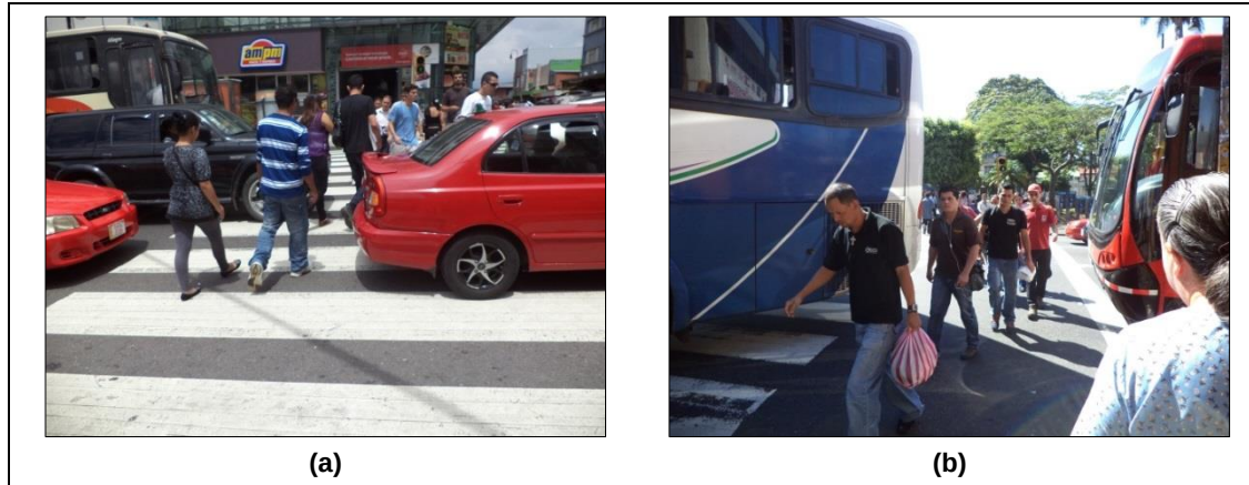
Figure 31: Conflict type MB: (a) Drivers fail to stop at stop line and enter crosswalk; (b) Buses queue in crosswalk while turning
