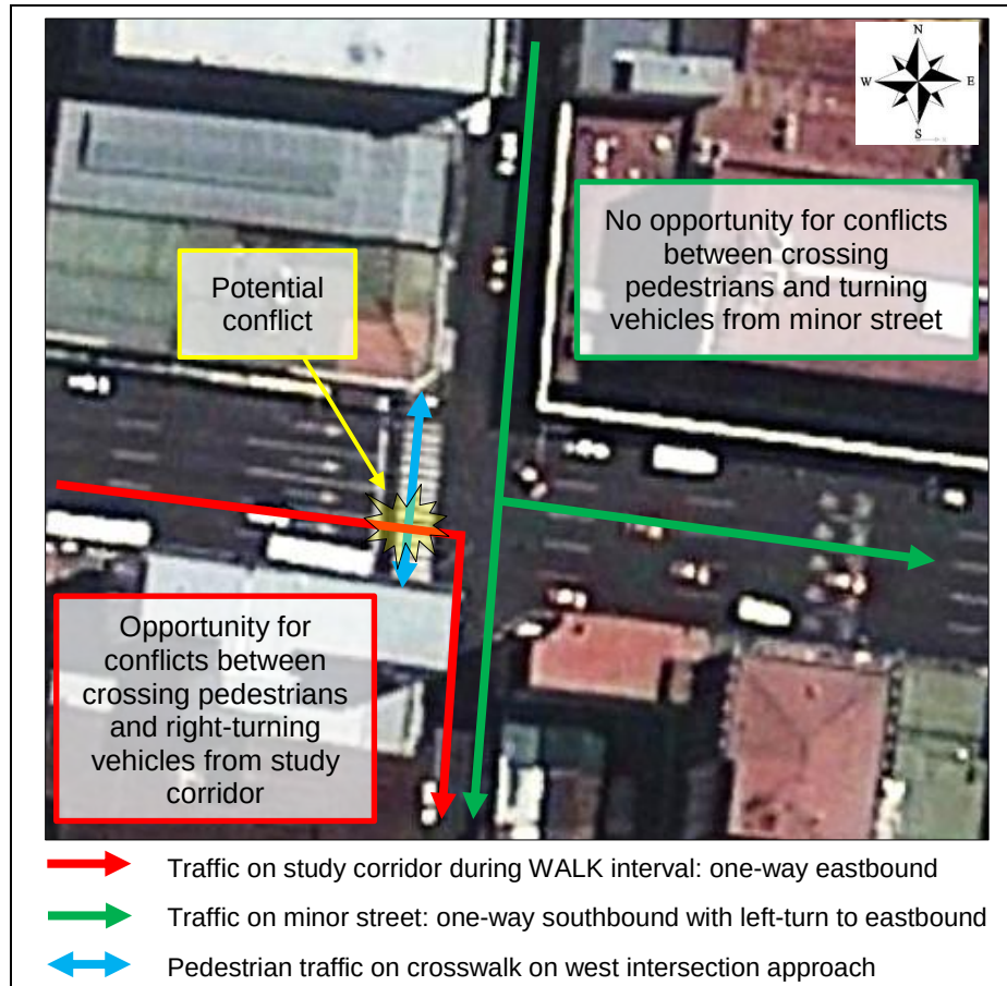
Figure 34: Conflict opportunity between turning vehicles and crossing pedestrians during the WALK interval at Site 10
